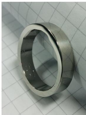
FIGURE 5.1: First amorphous wedding band made of  $\text{Pt}_{57.3}\text{Cu}_{14.6}\text{-Ni}_{5.3}\text{P}_{22.8}$  (85 wt% Pt).
