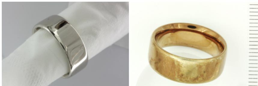
FIGURE 4.1: Color change of an amorphous ring with the composition  $\text{Au}_{49}\text{Ag}_{5.5}\text{Pd}_{2.3}\text{Cu}_{26.9}\text{Si}_{16.3}$  when worn for 52 days. Figure taken from Ref. [203].
