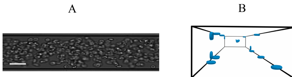
Figure 4.8. – A generic representation of a RBC suspension flowing through a microchannel. A A bright field image of a blood solution of 10% hematocrit level flowing in 60 \mu\text{m} wide microchannel; exposure time 3 ms, scale bar 30 \mu\text{m} . B Snapshot of numerical simulations showing margination of stiff RBCs in a rectangular duct channel. Normal red blood cells are omitted from the figure for clarity and as an analogy to experimental visuals.
