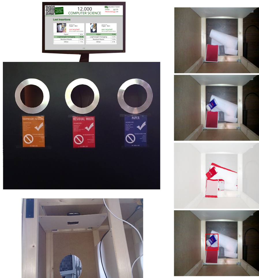
Figure 3.14: Trash can prototype of the Trash Game : Left: Exterior/interior. Right: Image extraction algorithm from top to bottom: before insertions; after insertions; recognized differences; rectangle showing extracted picture.
