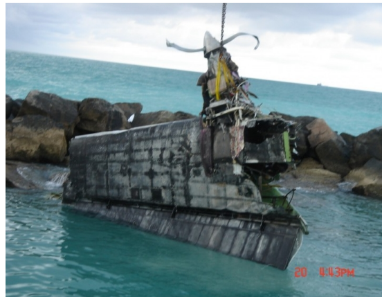
Figure 1.1 Separated wing of Grumman G73T aircraft ( www.skybrary.aero )
