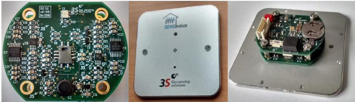
Figure 17: Sensor system prototype; Left: PCB with gas sensor / pre-concentrator device mounted in the middle; Center: aluminum flush-mount front panel with gas access; Right: fully assembled system ready for installation [232].
