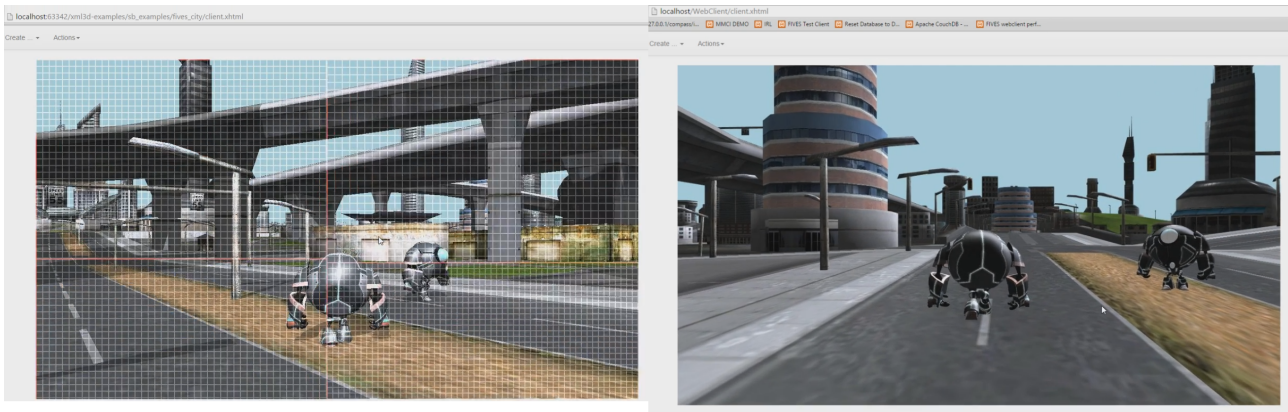
Figure 6.6: Two users explore a shared world in an example application running on top of XML3D and the distributed rendering framework. The server-side ray-tracer generates the left view, while the client-side WebGL rasterizer produces the right one. The tiling visualizes the server-side task distribution. The red lines show the distribution among four rendering nodes as determined by the cluster-level static load balancer. The white lines show the small tasks that the renderer uses on each node for the thread-level work stealing load balancer.
