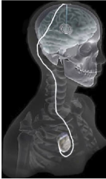
Figure 3.1: Overview of the DBS system. The DBS electrode is implanted in the brain during stereotactic surgery. The electrode is attached via an extension wire to the IPG, which is implanted in the torso. The entire system is subcutaneous and designed to deliver continuous stimulation for several years at a time.
