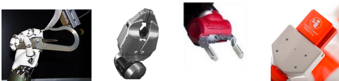
Figure 5.3: End-effectors on different robots, from left to right: dexterous hand on NASA’s robonaut, PR2’s jaw gripper, Baxter’s parallel plate gripper and UBR1 parallel jaw gripper
