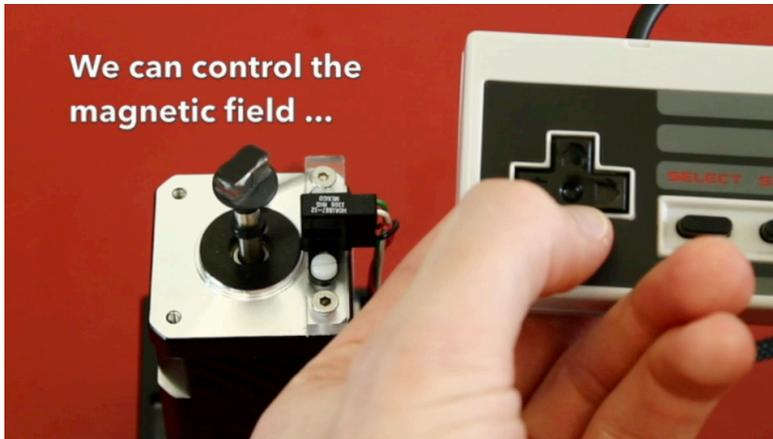
FIGURE 6.3 – *The stepper motor that controls the magnet direction is connected to a computer with a game console control. This allows for manual control of the propulsion of a single bacterium.*
