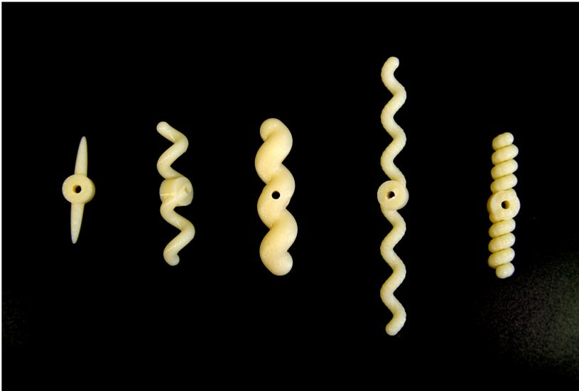
FIGURE 2.2 – Different shapes of models (from left to right): prolate spheroid, high helicity, high width, great length and high number of windings per length unit.
