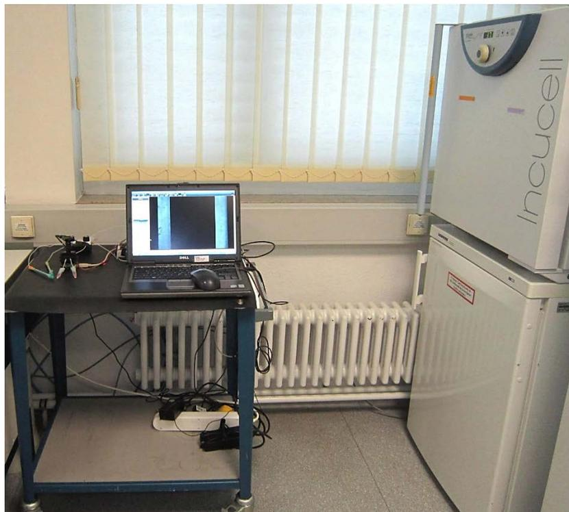
**Figure 4.4.2** Photo of the practical stand-alone cell culture and shadow imaging experimental setup, comparing to the bulky conventional incubator on the upper right of the photo. The whole experimental components are placed on a roll trolley. Real-time imaging of the dual-channel is showing on the screen of the laptop, which is very intuitive for the operator.
