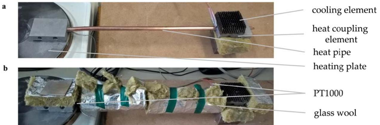
Figure 3.8: a) test bed showing the heat source (heating plate), the heat coupling elements on both sides with the heat pipe between them, the cooling element as well as the two temperature sensors (PT1000); b) test bed as in a), though completely coated with glass wool [NeFr2017b].
