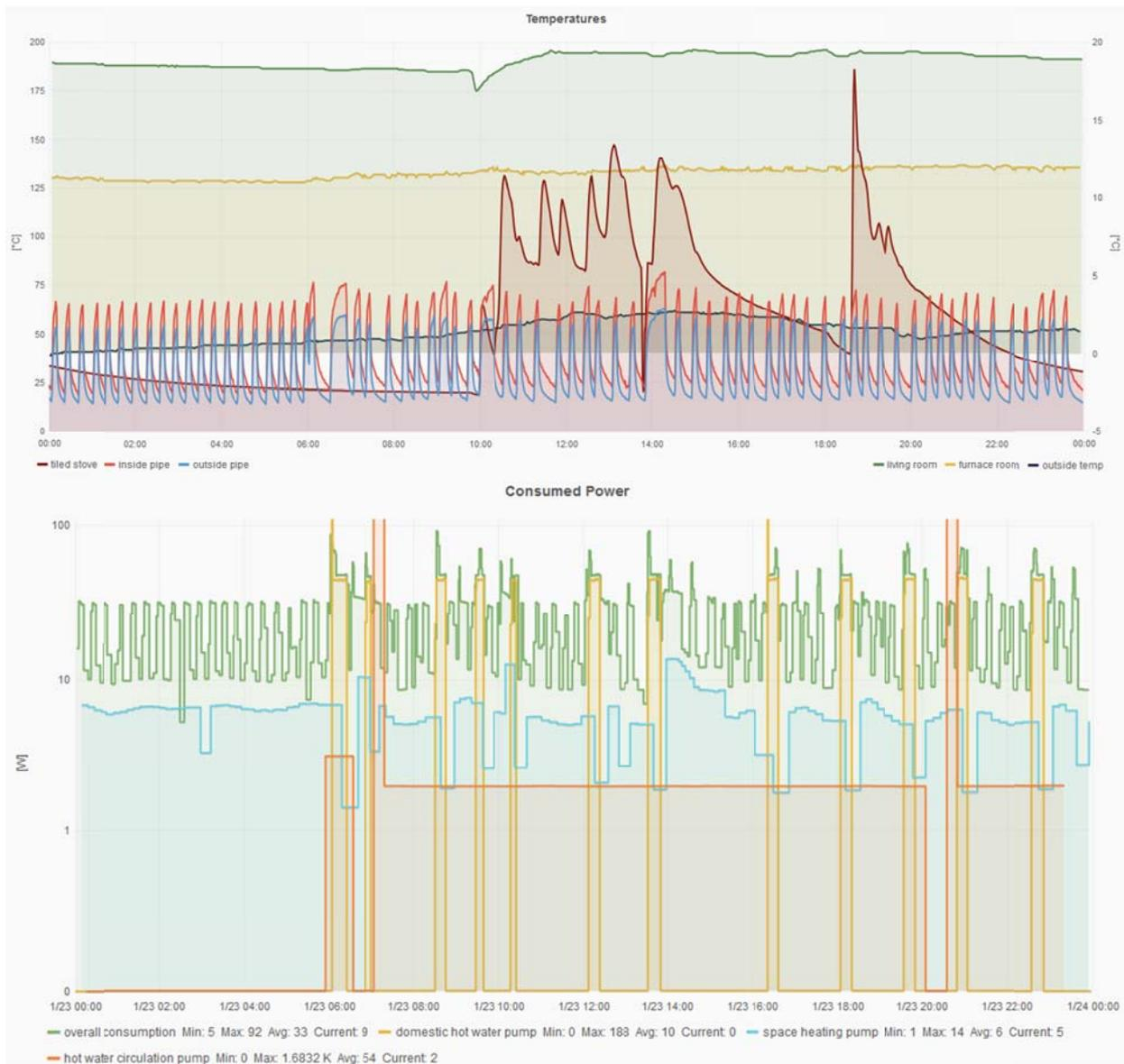
Figure 6.14: Measured temperatures at a heater and a tiled stove in a private house as well as power consumption of the pumps in the heating, illustrated by the web interface.
