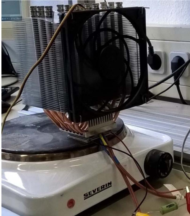
Figure 4.6: Experimental set-up to measure in a first round the open circuit voltage of a thermoelectric device and in the next step the generated electrical power. A heating plate serves as heat source and a CPU-cooling element as heat sink [NeFr2016a].
