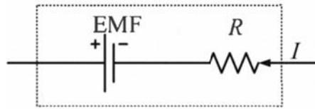
Figure 5.6: Equivalent circuit diagram of a TEG [Ch++2011].
