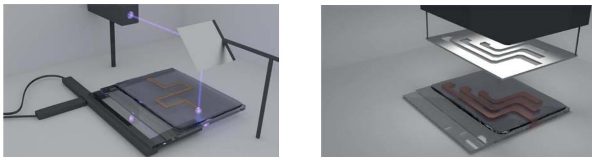
**Figure 40:** Schemes of techniques that can be implemented with different light sources **A.** direct laser writing **B.** photolithography.
