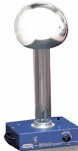
*Figure 1.13: (Left) Schematic diagram of Van de Graaff generator. Major components of VDG are two pulleys, two combs and rubber belt which can be driven by AC motor. Metal sphere can be a capacitance for electrons and it makes very high electric potentials. (Right) commercial VDG which can generate up to 350kV with 10 $\mu$ A constant current.*
