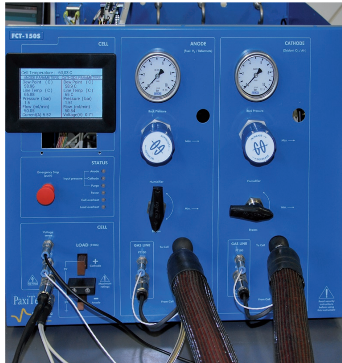
Figure 13: Test station system built during PhD duration. It contains on the front side all necessary connections to link a single PEMFC or a small stack.
