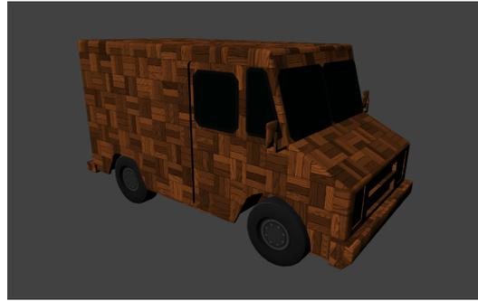
(b) Instantiation of the same asset, but overriding the material of the chassis geometry with a procedural shade.js material.
