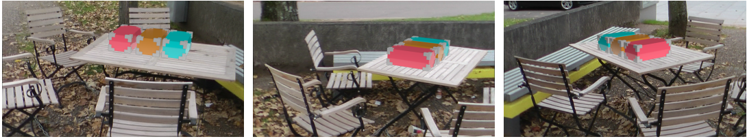
Figure 2.1: Three images of a real image sequence consistently augmented with virtual objects. The virtual camera path and scene geometry corresponding to the real image sequence were reconstructed with SfM. This information was then used to place three virtual boxes in the virtual scene. Finally, renderings of the virtual scene were generated and composited with the real images. Due to the accurate estimation of the camera position and orientation, the virtual objects are consistently positioned on the real table.
