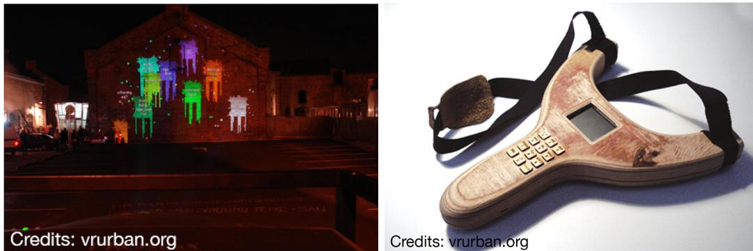
Figure 2.11: The SMSlingshot installation. Left: The media facade displaying user-generated content. Right: The SMSlingshot device [55]. A user can shoot a message onto a facade by aiming at a specific point with the slingshot.
