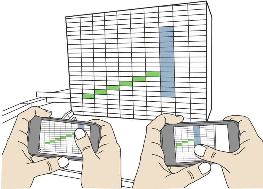
Figure 4.2: Allowing multiple users to simultaneously interact with a media facade through live video on mobile devices. Manipulations by all users on the mobile device are immediately displayed on the facade. The colors denote actions of different users.
