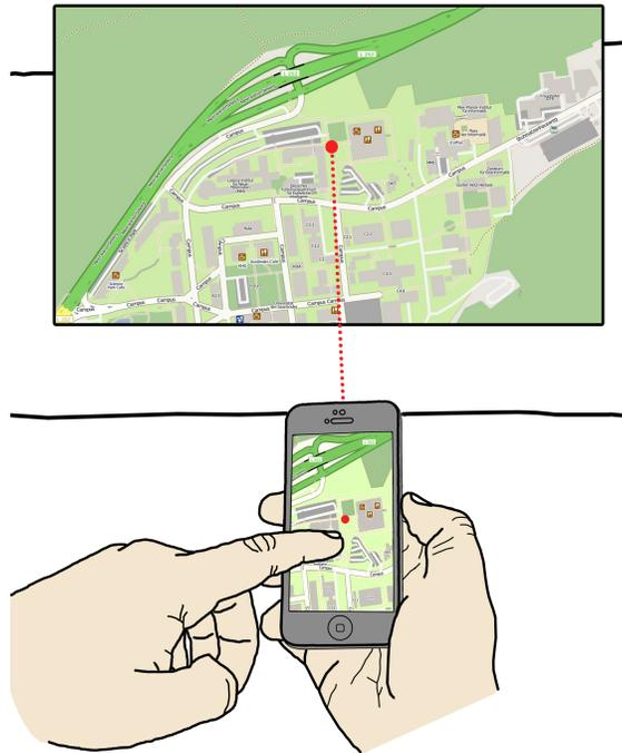
Figure 4.10: Pointing at a display with a mobile device. The content around the current pointer position on the display is displayed as a preview on the mobile device’s screen, with which the user can interact by direct touch input. The current pointer position (red dot) is displayed on both the mobile device and the remote display.
