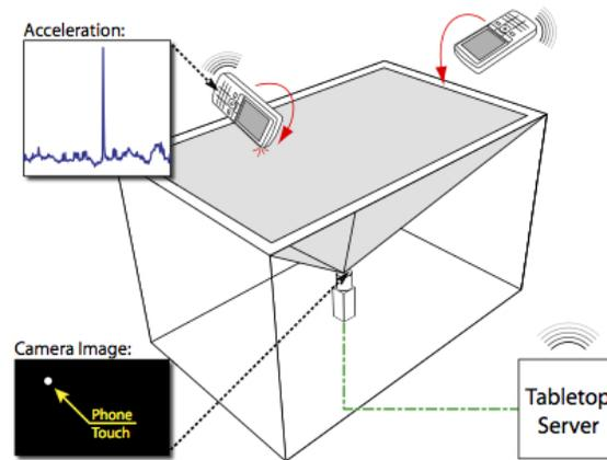
Figure 2.18: Touching a surface with mobile phone using PhoneTouch: Surface and phones independently detect the touch events and communicate the observations over a wireless network, correlated in time, and combined to associate a touch with both surface position and phone identity [159].
