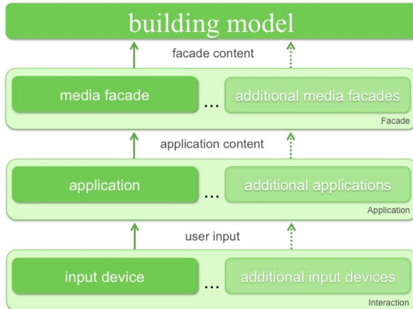
Figure 5.5: The structure of the toolkit. The building model, media facades, applications and input devices are organized in separate modules, retaining a flexible structure. Communication takes place only between pairs of modules. Input devices send user input to the applications, the applications communicate their visual content to media facades and they communicate the facade content to the building model.
