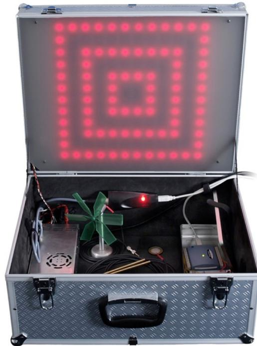
Figure 5.3: Pre-testing design concepts using Lightbox [193], a mobile prototyping toolkit to simulate the hardware interplay of interactive media facade installations.
