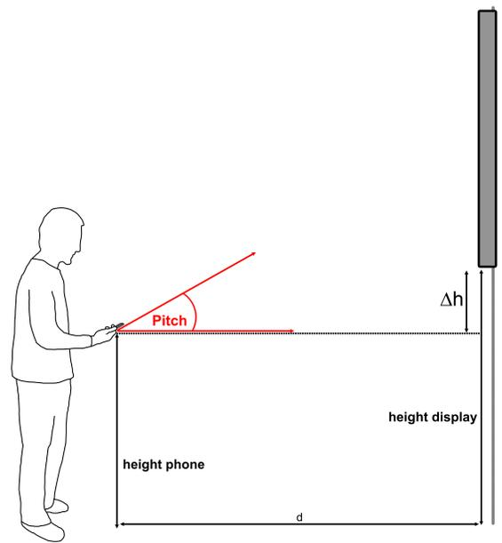
Figure 4.11: Calculating the vertical intersection of the current pointing direction and the vertical display area.
