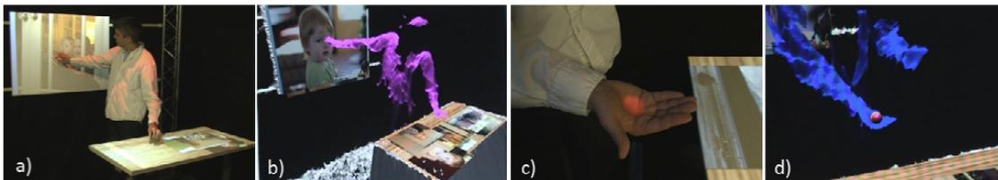
Figure 2.16: The *LightSpace* prototype combining depth cameras and projectors to provide interactivity on and between surfaces, including object transitions through-body between existing interactive surfaces (a-b), as well as interactions with an object in hand (c-d) [198].
