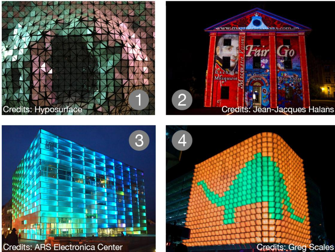
Figure 3.1: Four categories of media facades: (1) Mechanical facade, (2) projection facade, (3) window raster animation facade and (4) illuminated facade.
