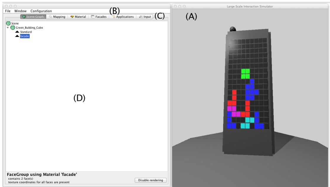
Figure 5.13: The interface of the media facade toolkit: (A) the rendering view, (B) the control view, (C) control groups and (D) the detailed settings.
