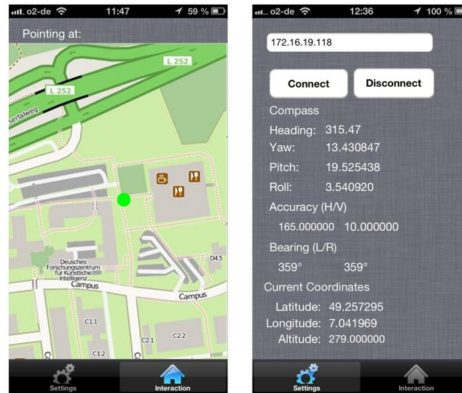
Figure 4.13: The interface of the mobile client prototype. Left: The detail view displaying the content around the current cursor position. Right: A settings view, displaying the current sensor data, utilized for calculating the cursor position.
