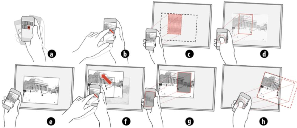
Figure 2.22: Virtual Projection [12]: (a) Shaking the device to create a view. (b) Interacting with a non-projected view. (c-e) Creating a projection by aiming at the secondary display, pressing and holding, and releasing. (f) Synchronized interaction. (g) Projection frustum can be used for filtering or navigating. (h) Projections can be moved or deleted by aiming, pressing and holding, and dragging out of the display [12].
