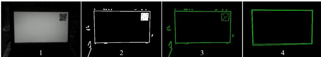
Figure 4.6: Detecting a distant display: (1) Converting the image into a gray-scale image and applying Erosion. (2) Applying Canny Edge Detection and Dilation. (3) Verifying contours. (4) Finding the rectangle nearest to the center of the image.
