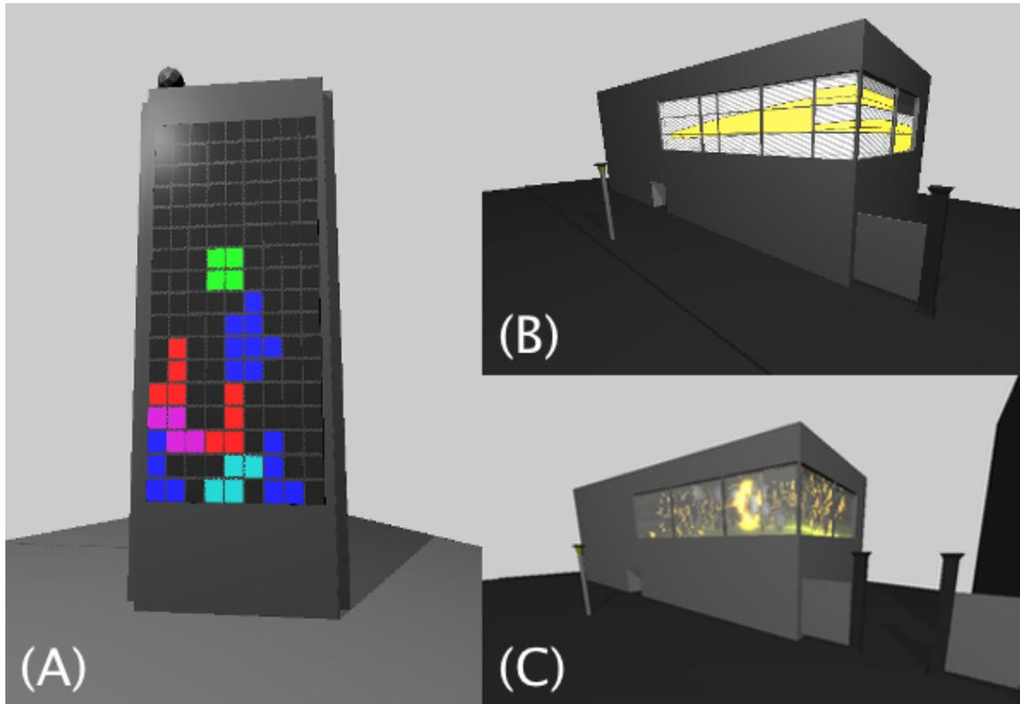
Figure 5.14: Applications developed using our toolkit. (a) Tetris: This game was developed as a standalone application and simulated on differently shaped facades. (b) Move-the-tile: A multi-user puzzle. The application was developed using the facade toolkit throughout the design process. (c) A video player to display videos and animation on various media facades.
