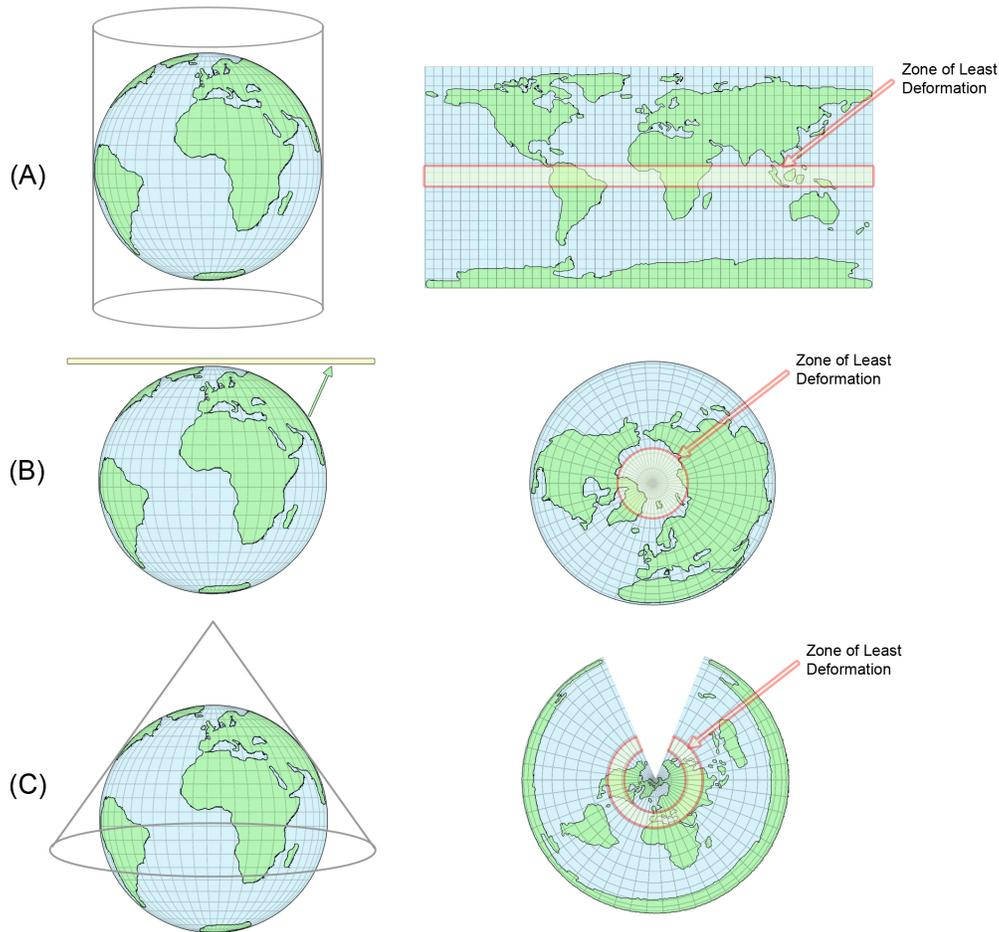
Figure 4.18: Characteristic map projections with different projection surfaces and the area of least deformation: (A) cylindrical projection, (B) azimuthal projection, (C) conic projection.
