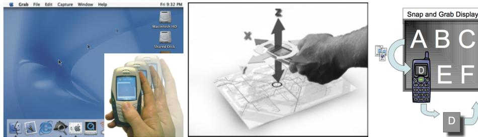
Figure 2.19: Left: Controlling a pointer with the *Sweep* technique [5]. Middle: Calculating a mobile device’s position and orientation to a remote display with 6 degrees of freedom using computer vision [85, 84]. Right: Transferring multimedia content over Bluetooth applying the *SnapAndGrab* technique [120, 119].
