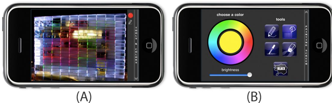
Figure 4.5: The interface of the painting application. To keep the drawing canvas as large as possible (A), users can switch to the tool palette (B) by performing a sliding gesture.
