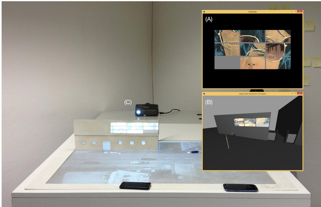
Figure 5.12: Using the toolkit’s hybrid simulation feature to display the application simulated with the toolkit onto a physical miniature model of the media facade. (A) The view of the toolkit’s external camera. (B) The virtual simulation of the facade. (C) Projecting the toolkit’s external camera view onto a physical miniature model.
