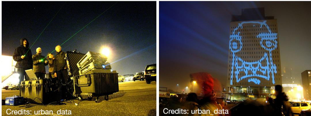
Figure 2.12: Left: The technical setup of the Laser Tag installation, comprising two projector for creating the media facade. Users are interacting by pointing at the facade with a laser pointer whose movement is tracked by a camera. Right: Content created by users.
