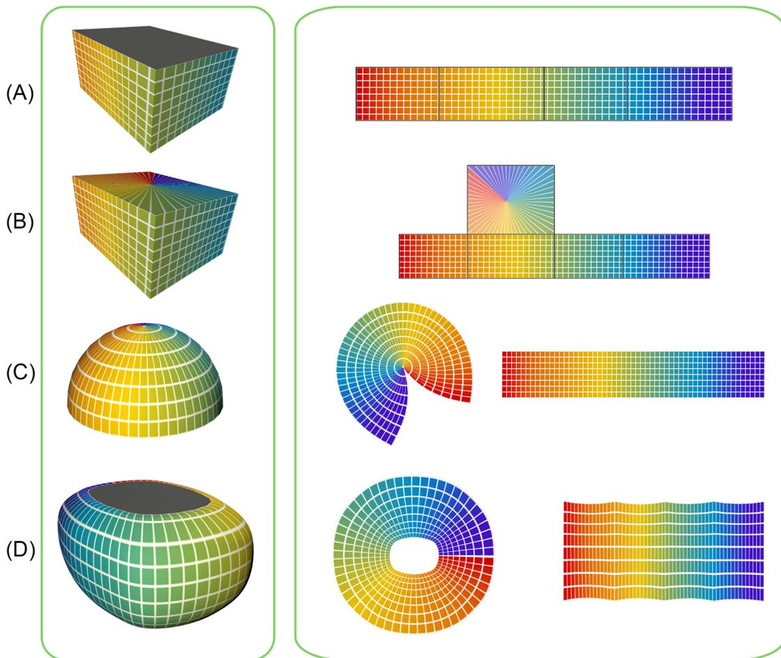
Figure 4.19: Map projections for different building shapes. (A),(B) Cubic form factor: cubic projection. (C) Spherical form factor: (left) conic projection, (right) cylindrical projection. (D) Curved form factor: (left) azimuthal, (right) cylindrical projection
