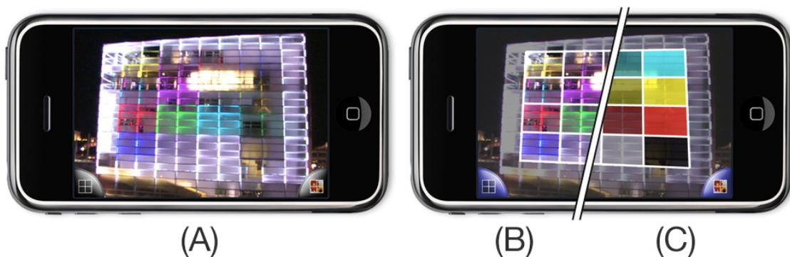
Figure 4.4: An interactive puzzle application displayed on the facade. On request, the original video image (A) is augmented with a grid (B) to determine the tiles or a preview of the solved puzzle (C).
