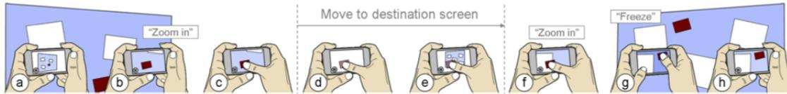
Figure 2.21: Moving content between displays using *Touch Projector* [23]: (a) the user aims at a display (b) causing the device to automatically zoom in. (c) This allows the user to touch the red target object and (d) hold it while turning the device towards the other display. (e) Once the device detects the secondary display, (f) it zooms in again. (g) Pushing the freeze button causes the live camera image to pause for precise manipulation. (h) Lifting the finger releases the object [23].
