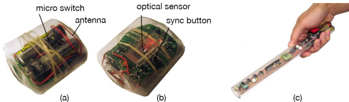
Figure 2.17: (a),(b): Top and bottom view on the core component of Soap [10]. (c): The XWand device [197].
