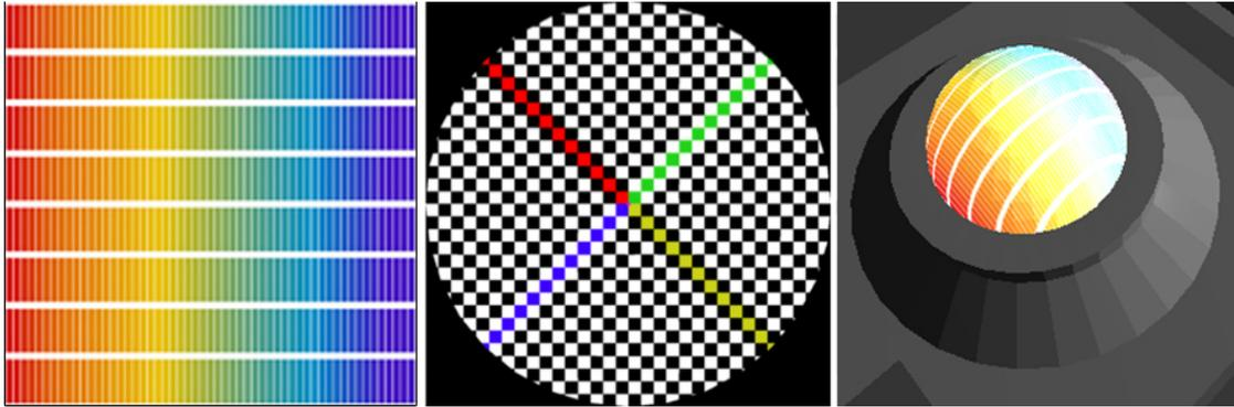
Figure 5.9: Mapping an application onto a media facade model as a texture. To get a better impression of the mapping and the introduced distortion, the texture shows a test image rather than an actual application. Left: the texture image to be mapped onto the model. Middle: The 2D image created from the 3D model surface by applying map projections. Right: The texture image mapped onto the 3D model.
