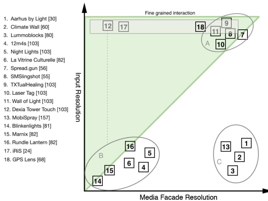
Figure 4.15: Placement of the introduced interaction technique (GPS Lens) in the classification (see also Section 3.2.1) by input and media facade resolution (18). Although initially developed for high-resolution facades, it is also applicable to various resolutions.
