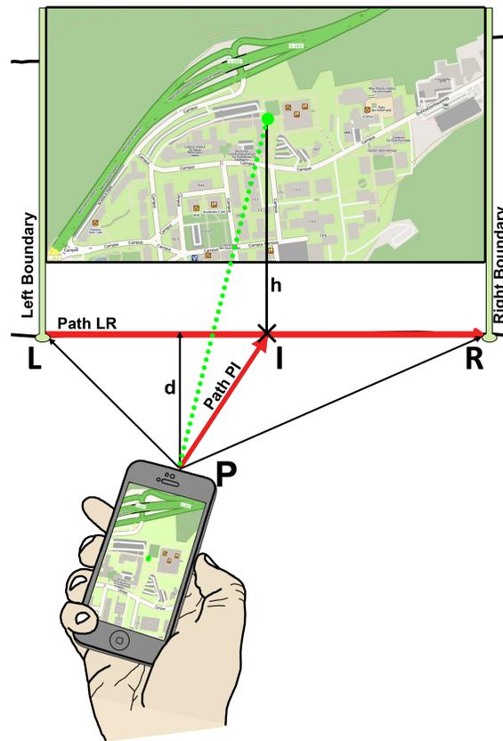
Figure 4.12: Calculating the horizontal intersection of the current pointing direction PI and the display area.
