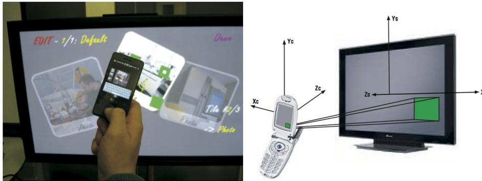
Figure 2.20: Left: Images being moved, rotated and scaled using the display registration by Pears et al. [144]. Dynamic visual markers are displayed around the particular content elements. Right: The geometry of a smart phone viewing a marker on a public display [144].
