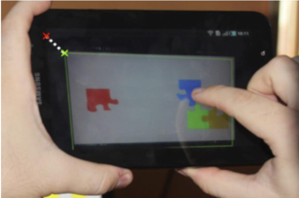
Figure 4.7: A detected display (green rectangle). The red x denotes the zero point of the touch-capable area. The green x denotes the zero point of the coordinate system, which is used for mapping the touches.
