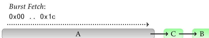
Figure 4.4: *LEON2 Timing Anomaly*: The example demonstrates a timing anomaly present in the LEON2 processor caused by the instruction cache line fill mechanism. The basic blocks A, B, and C reside in the same cache line. The local best-case – assuming a cache hit for the instructions in basic block A – causes the global worst-case execution of the example: The core performs ten instructions fetches. On the contrary, only eight instruction fetches are issued upon an initial cache miss.
