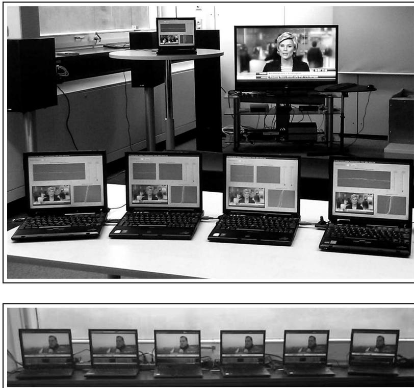
Figure 10.7: Prototype implementation used for local DVB-T redistribution to a group of receivers. *Top*: A leader receiver (top left) is placed deliberately further away from the base station (behind the camera); live DVB-T is shown on a TV set for comparison (top right). *Bottom*: All receivers are placed deliberately close together; the leader is randomly chosen and uses feedback power reduction.
