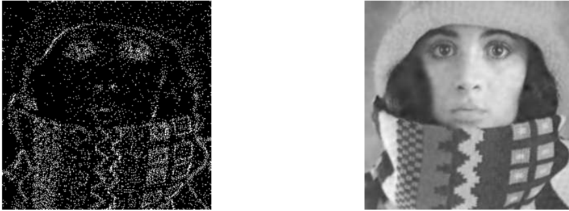
Figure 3.26: Biharmonic inpainting for trui . (a) Left: Inpainting mask with 10% specified pixels. (b) Right: Reconstruction with biharmonic inpainting (explicit scheme, T = 1000000 , \tau = 0.025 ).
