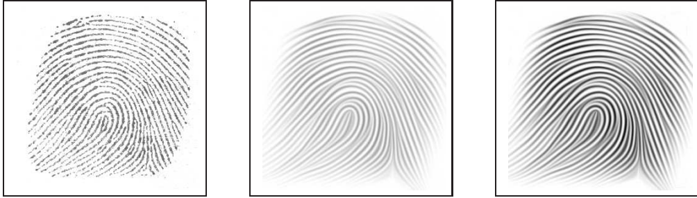
Figure 3.22: Fingerprint enhancement with CED. (a) Left: Original image ( 300 \times 300 ). (b) Middle: Filtered with the semi-implicit scheme ( \tau = 0.05 ) using the model parameters \lambda = 1 , \sigma = 1/2 , \rho = 4 , \alpha = 10^{-3} and stopping time T = 300 . (c) Right: Rescaled to [0, 255] for better visualisation.
