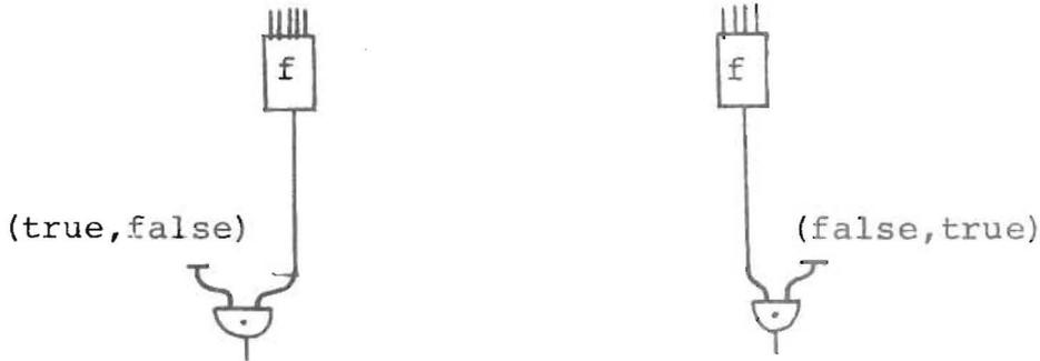
Then  $\|f_1\| \geq |f'| = \|f\|$  and  $\|f_2\| \geq |f'| = \|f\|$ . On the other hand  $f_1 * f_2$  may be computed using the following switching circuit:
