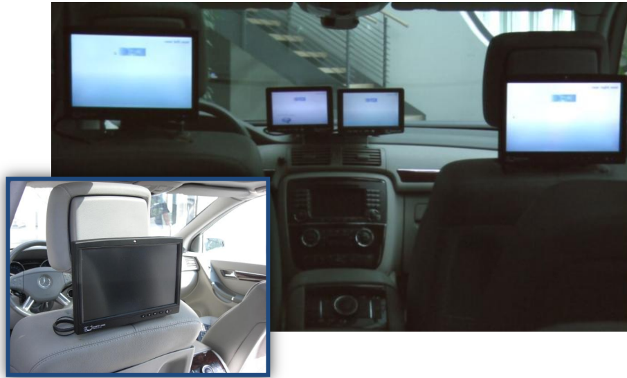
Figure 6.17: Instrumentation of each seat in the demonstration vehicle with a screen and integrated microphone.
