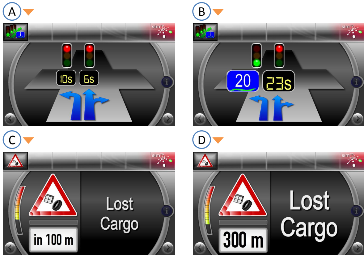
Figure 6.15: Functions adapted to decreased sight / visual impairment. (A) Traffic light phase assistance function with normal font size (note that not all possible slots for traffic lights have been used). (B) The same function with the adapted layout using larger fonts at the cost of clarity and number of possible traffic lights. (C) Non-adapted obstacle warning screen showing the type of obstacle and distance. (D) Adapted obstacle warning featuring larger fonts at the cost of maximum text length (which for this warning is not a problem).
