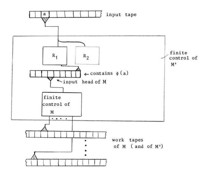
If  $R_2$  has determined that the input is in K the input head is reset to the beginning of the input and M' works in the following way: The finite tape in the finite control will contain  $\phi(a)$  if a is the symbol just read by M'. If M''s input head is going to leave this tape at its right (left) border R will produce  $\phi(b)$  where b is the symbol right (left) from a in the input.
