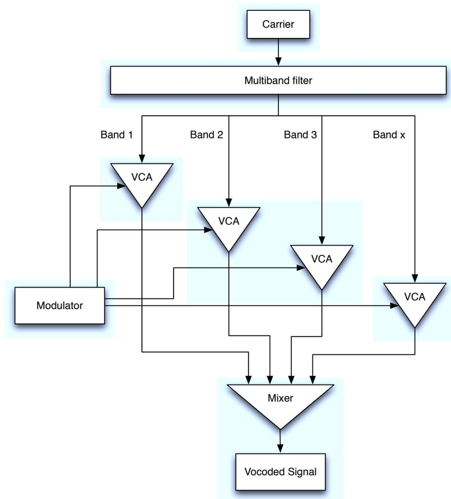
**Figure 6.2:** The vocoding principle<sup>1</sup>
