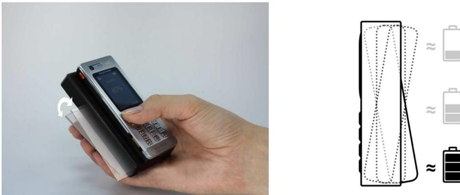
**Figure 3.35:** Left: The shape changing phone prototype - Right: A battery status indicator (source: [Hemmert et al., 2010])
