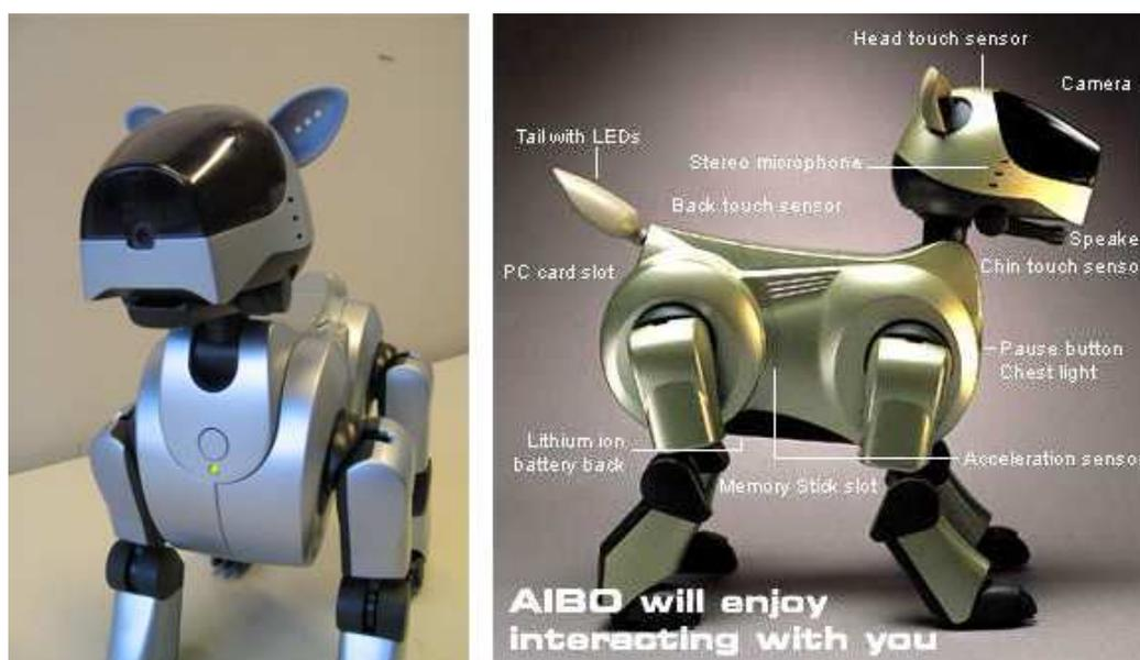
**Figure 3.42:** Sony's AIBO (sources: <http://commons.wikimedia.org/> and <http://www.robotstoreuk.com>)
