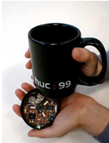
**Figure 3.2:** *The augmented MediaCup (source: [Beigl et al., 2001])*
