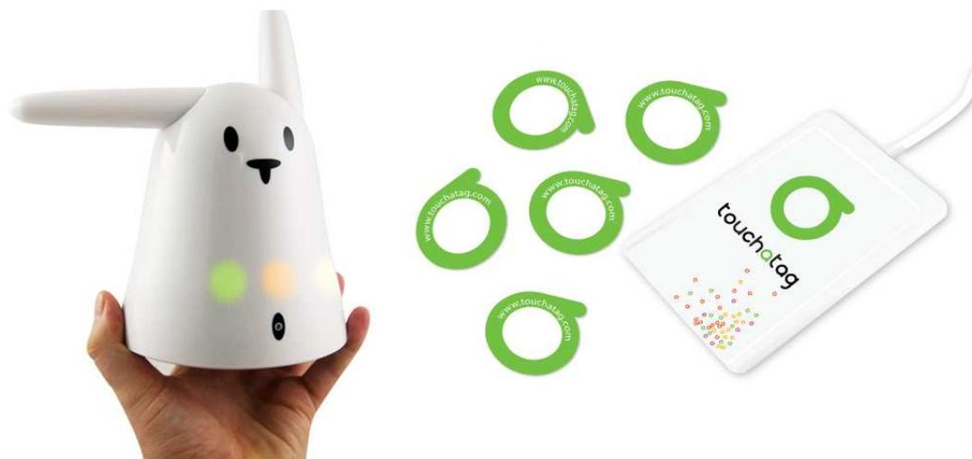
**Figure 3.7:** Left: The Nabaztag - Right: A Touchatag set incl. RFID reader and tags (sources: <http://www.violet.net/> and <http://www.touchatag.com/>)
