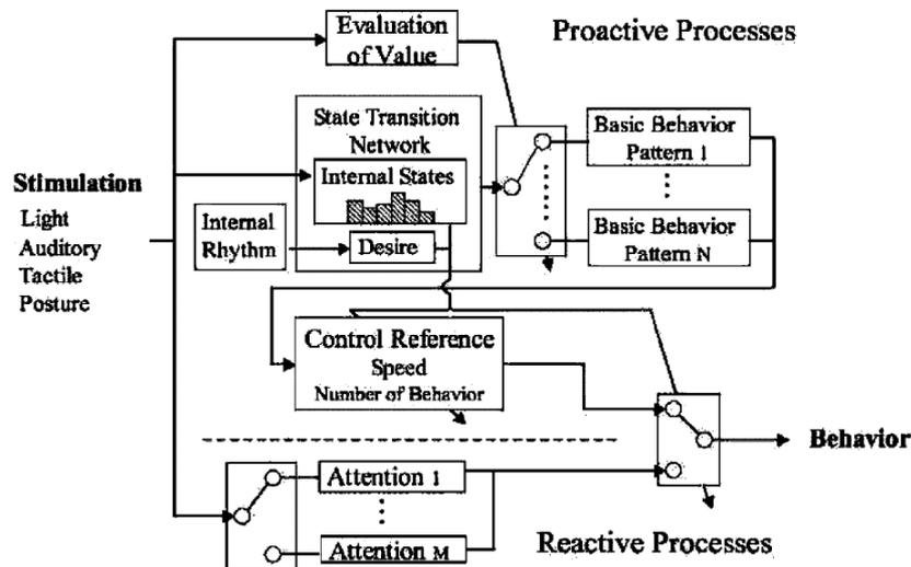
**Figure 3.38:** The behaviour generation system of the Paro seal robot (source: [Wada and Shibata, 2007])
