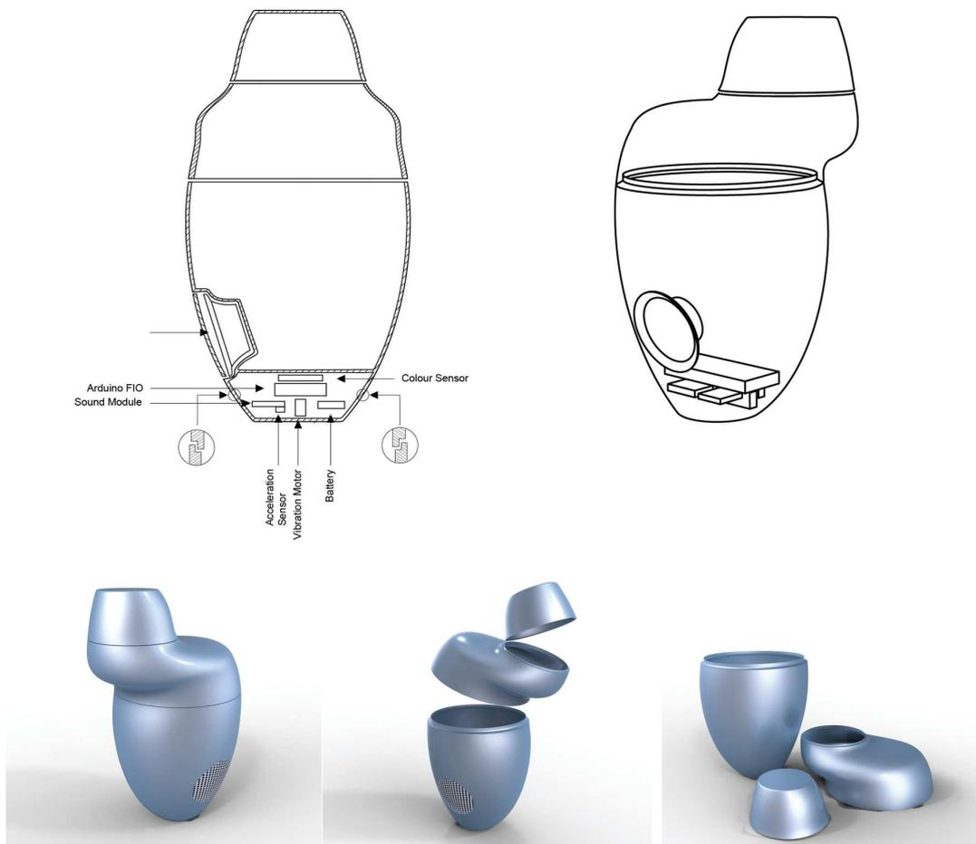
**Figure 8.14:** Technical drawings and 3D models of the shaker
