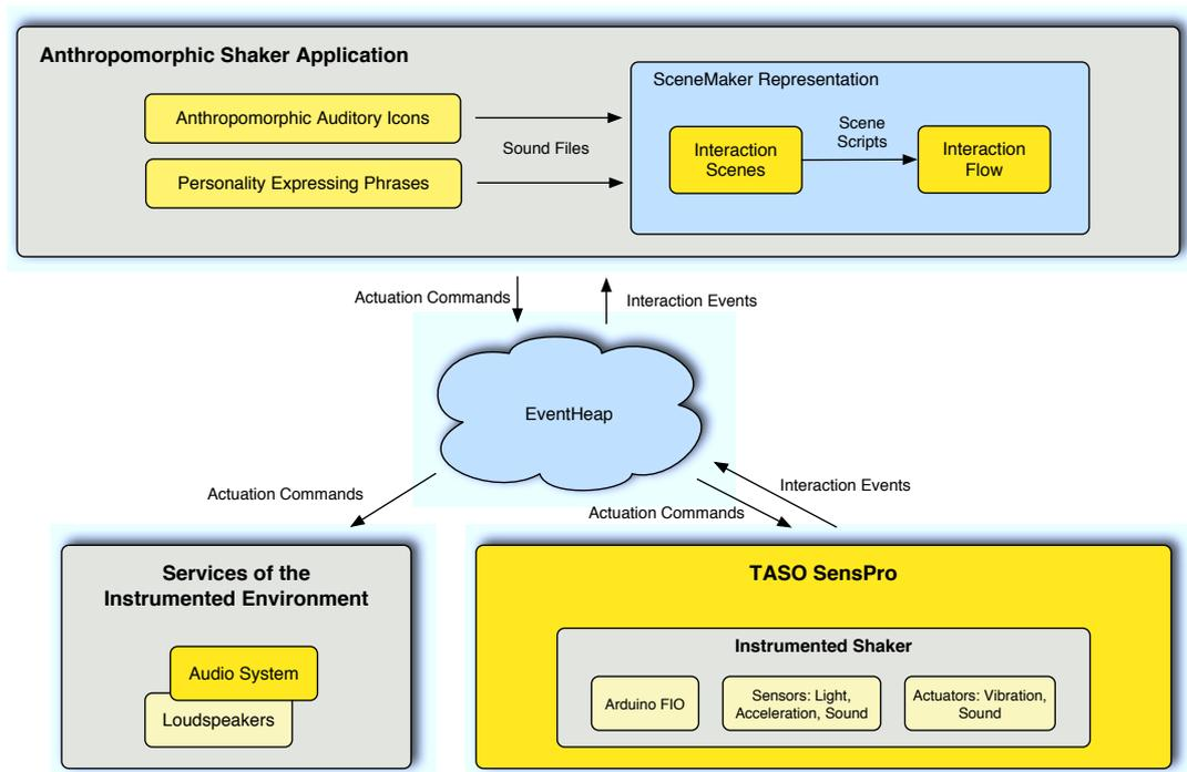
**Figure 8.13:** The overall architecture of the Anthropomorphic Cocktail Shaker based on the TASO Platform
