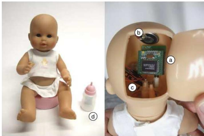
**Figure 3.8:** Integration of the Wireless Voice Node into the speaking doll: a) the Wireless Voice Node, b) loudspeaker, c) battery, and d) a milk bottle as smart toy (source: [Lombriser et al., 2009])
