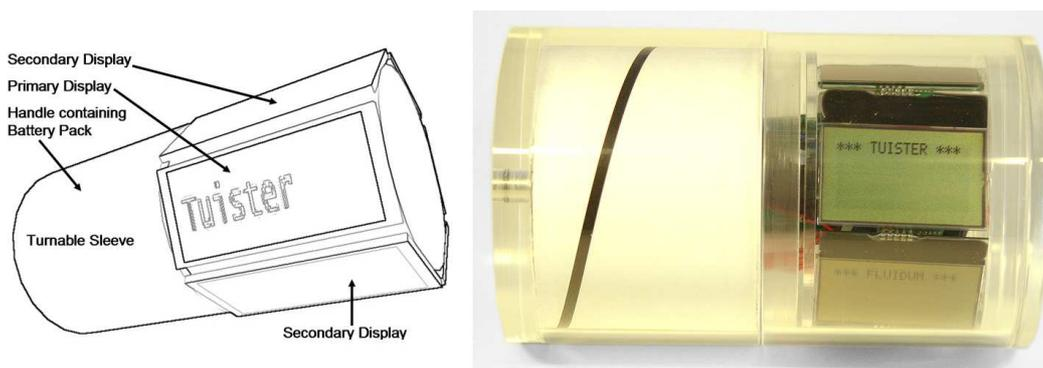
**Figure 3.12:** The Tuister design (left) and prototype (right) (sources: [Butz et al., 2004])
