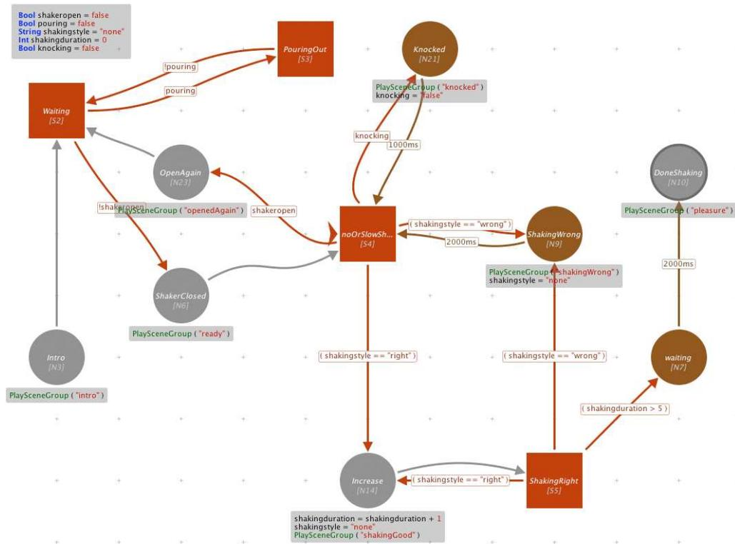
**Figure 8.10:** The top level of the scene graph for the anthropomorphic shaker
