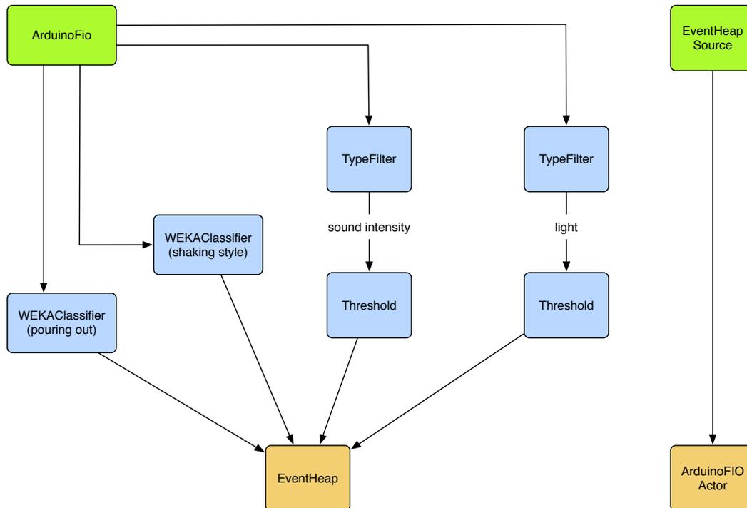
**Figure 8.12:** The sensor processing filter chain of the shaker
