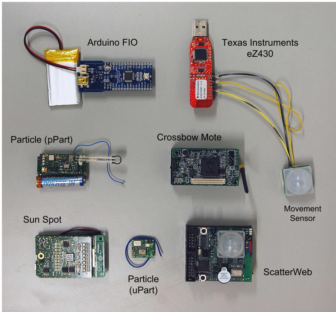
**Figure 5.1:** Sensor nodes experimented with during the development of TASO SensPro
