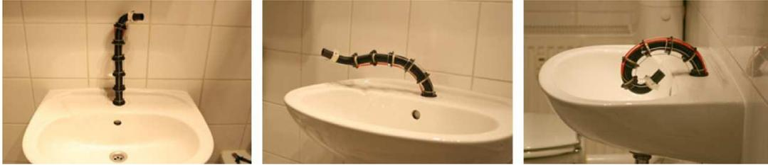
**Figure 3.29:** *The Thrifty Faucet in different postures: seeking, curious, rejecting. (source: [Togler et al., 2009])*
