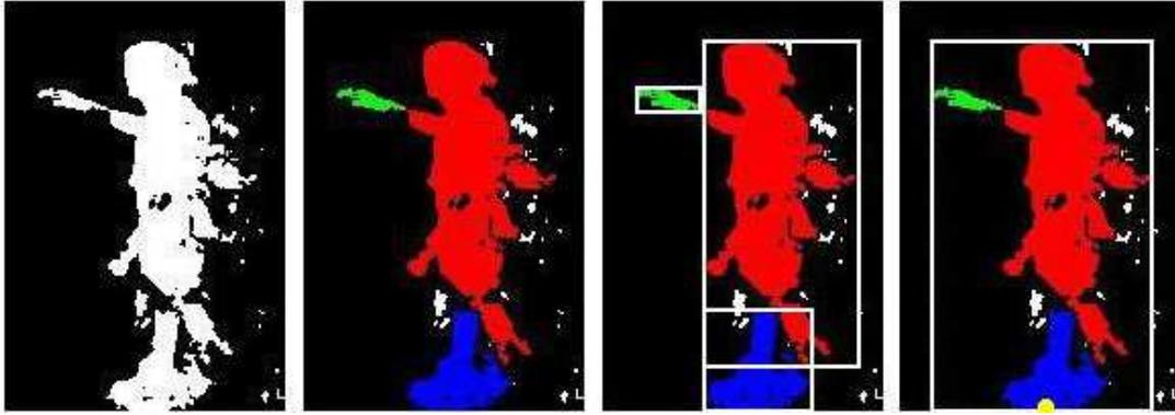
**Figure 5.7:** Region merging. From Left to Right: Part of motion image. Connected component labelling yields three non-negligible blobs (coloured). Assign one region per blob. Merged regions to one person region with tracepoint  $\mathbf{x}_t$  (yellow spot)
