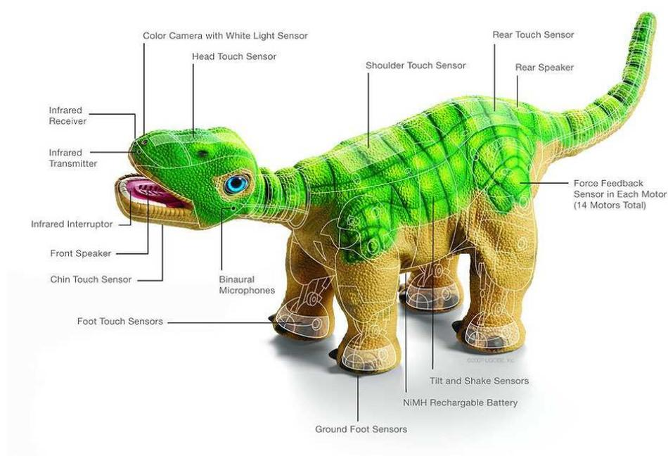
**Figure 3.43:** Placement of Pleo’s sensors (source: <http://www.pleouk.co.uk>)
