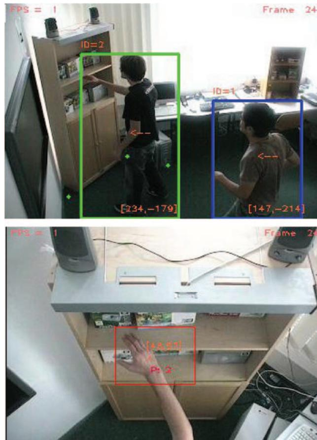
**Figure 5.8:** Macro-tracking: Person regions with position in world-coordinates, moving direction and ID (top). Micro-tracking: Skin region associated to person with ID 2 (bottom)
