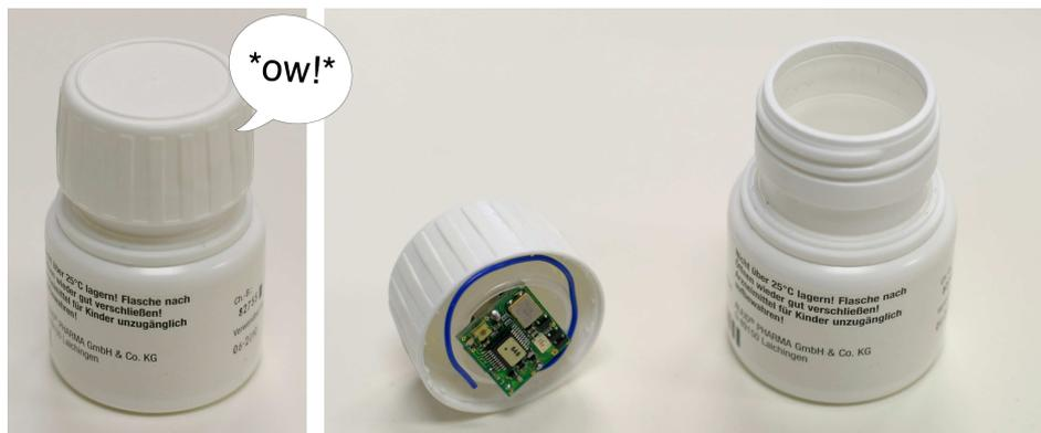
**Figure 8.1:** The Sensing Pill Box complaining when exposed to heat (left), the integrated sensor (right)
