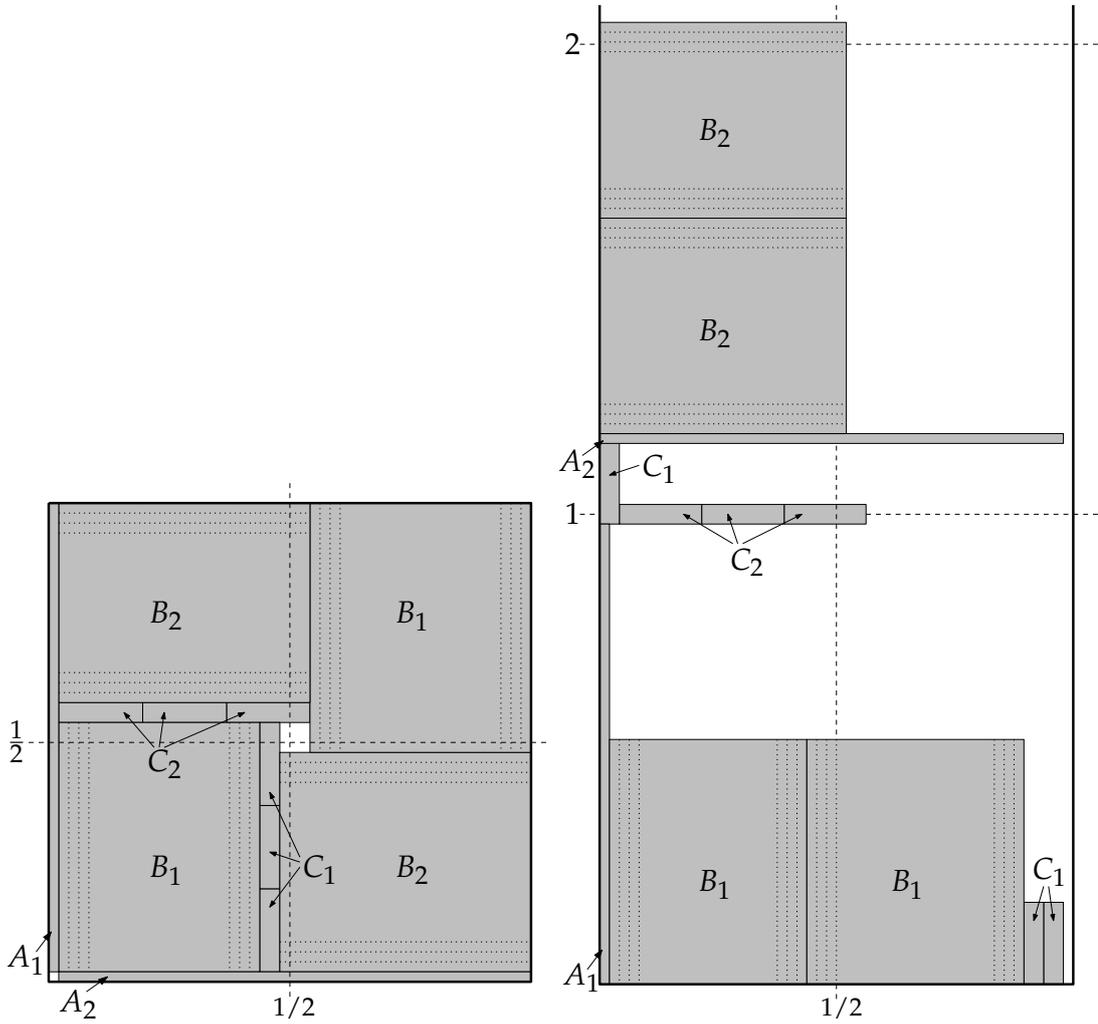
Figure 25: A lower bound instance for HFF. The left side shows that  $\text{OPT}(I) = 1$  whereas the right side shows the FFDH packing. FFD packs  $A_2$  together with the first layer into a bin. The remaining layers have total height greater than 1 and thus do not fit into a second bin.
