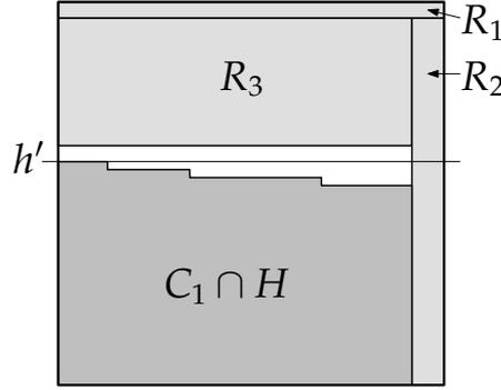
Figure 23: The three rectangles  $R_1$ ,  $R_2$  and  $R_3$  for packing  $T'$  together with  $C_1 \cap H$  in  $C_1$ .
