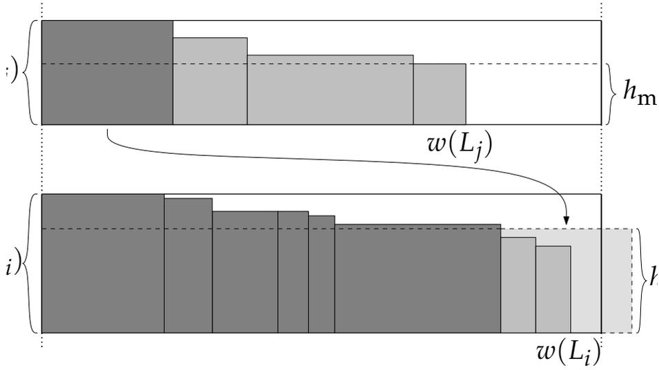
Figure 26: Deriving a bound for the volume in two layers. All items that are packed up to and including the first item in  $L_j$  are dark and have height at least  $h_{\max}(L_j)$ . The total width of these items is greater than 1. All other items have height at least  $h_{\min}$ .
