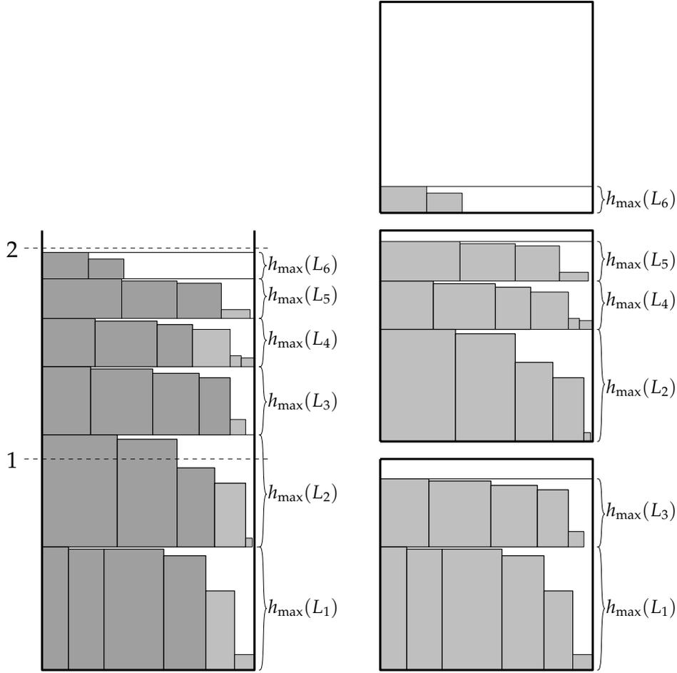
Figure 24: The HYBRID FIRST FIT algorithm. The layers of a strip packing with FFDH are packed into bins with FFD. Items that are placed into a layer after a new layer was opened are shown in light grey
