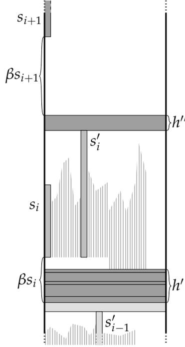
Figure 34: Packing after the  $(i + 1)$ -th jump. The blocking items that arrived after  $s_i$  are shown in darker shade. By definition,  $s_i$  is the first item that does not fit into the previous interval. Thus we have  $s_{i+1} > s'_i + \beta s_i - h'$
