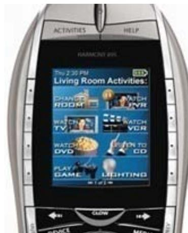
Figure 136: The activity-based Harmony universal remote control. Image: Logitech GmbH.
