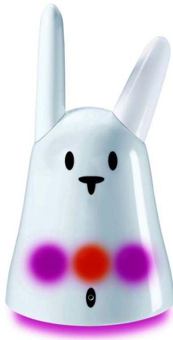
Figure 10: The *Nabaztag* rabbit is wirelessly connected to the internet and can communicate information to the user by moving its ears, flashing LEDs, reading messages, or playing music. Image: Wikimedia.
