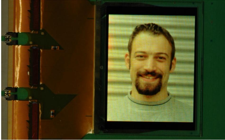
Figure 1.2: A demo board with an OLED display to test CMLA. The image is displayed using CMLA2.
