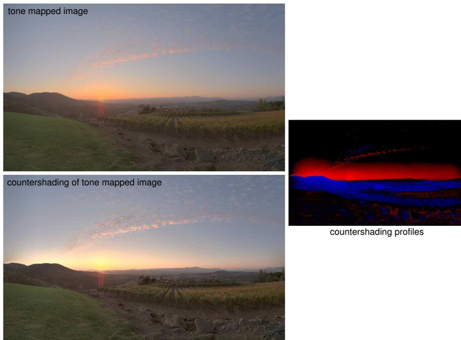
Figure 7.10: Image tone mapped using logarithmic mapping [Drago et al. 2003] (top) and restored using adaptive countershading (middle). Subtle changes to the image bring back the contrast at the horizon and the details, but do not change the style of the image. Image courtesy of SpheronVR.
