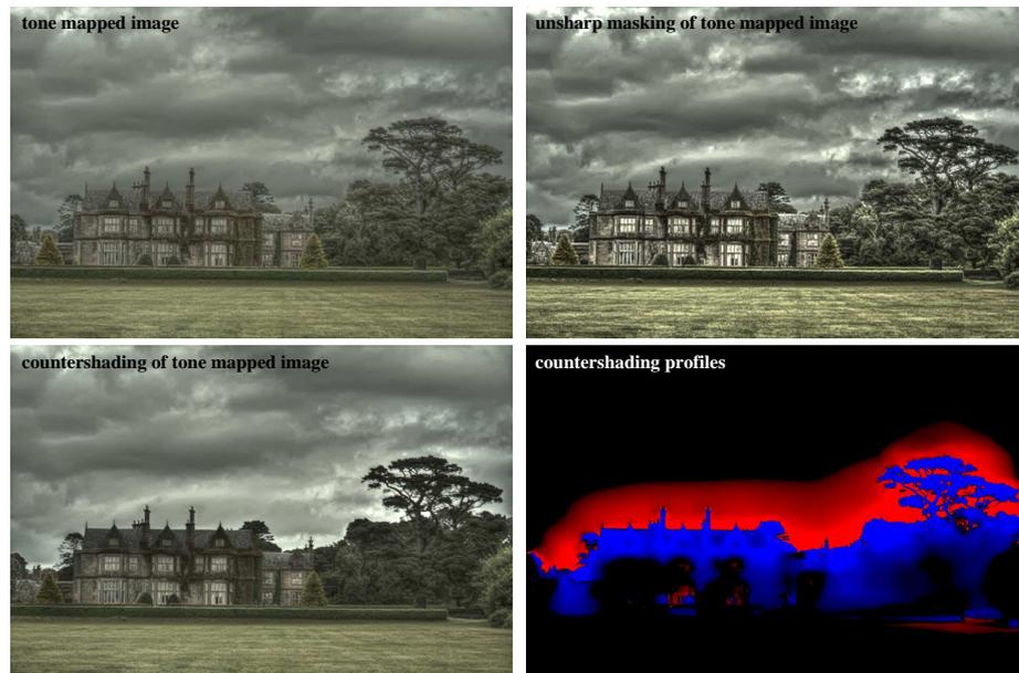
Figure 7.9: Image tone mapped using the contrast equalization [Mantiuk et al. 2006] (top/left) and restored by adaptive countershading (bottom/left). The restored image better communicates the brightness relations and the depth in the image. (top/right) shows unsharp masking with parameters set manually to equal dominant countershading profile. Although overall enhancement of unsharp masking is impressive, the changes are hardly controllable and modify the style of the image.
