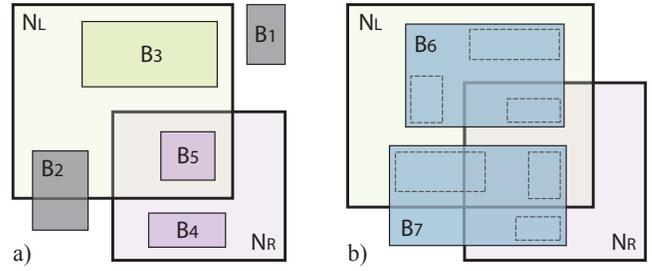
**Figure 4:** Accept and reject tests for the cost calculation. a) Nodes  $B_1$  and  $B_2$  would reject the configuration. All primitives of  $B_3$  are put into  $N_L$  and the primitives of  $B_4$  - into  $N_R$ .  $B_5$  is put into the child with smaller surface area ( $N_R$  in this case). b) Undecided cases: the nodes of  $B_6$  and  $B_7$  cannot be uniquely assigned neither to  $N_L$  nor to  $N_R$ . The algorithm needs to refine them recursively.
