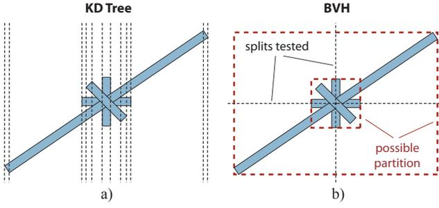
**Figure 1:** An extreme case where the centroids of all objects in a node coincide. While KD tree construction will be able to partition the set, classic BVH construction will have to create a leaf node, even though it would be more optimal to create two children nested in each other.
