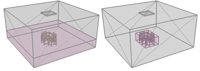
**Figure 2:** A partition of the root node of the SHIRLEY6 scene produced by the classic BVH partitioning algorithm (left) and our geometric partitioner (right). Note that the classic algorithm has also created nested siblings.
