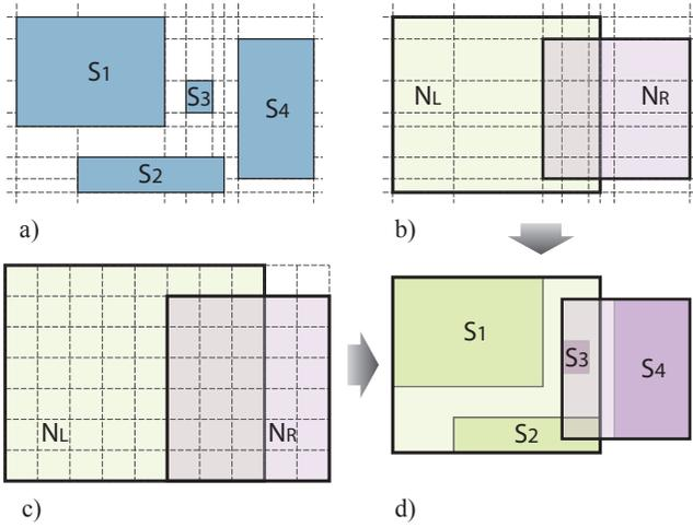
**Figure 3:** Geometric partitioning. a) The set of objects. b) Candidate AABBs picked at object boundaries. c) Candidate AABBs picked on a grid. d) Objects fully contained in both AABBs are put into the one with smaller surface area, and bounds are tightened.
