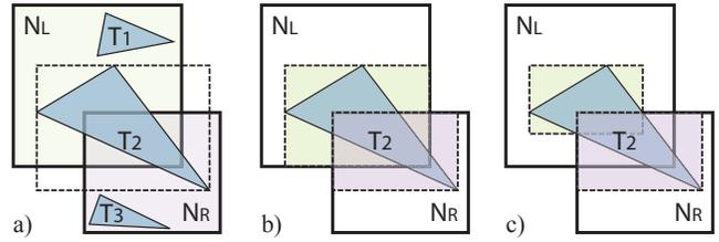
**Figure 5:** Triangle splitting. **a)** A configuration is feasible iff the geometry is covered by the children's AABBs. **b)** A triangle can be split by clipping it to the child AABBs or **c)** by clipping it to the child with smaller area and putting what remains in the other.
