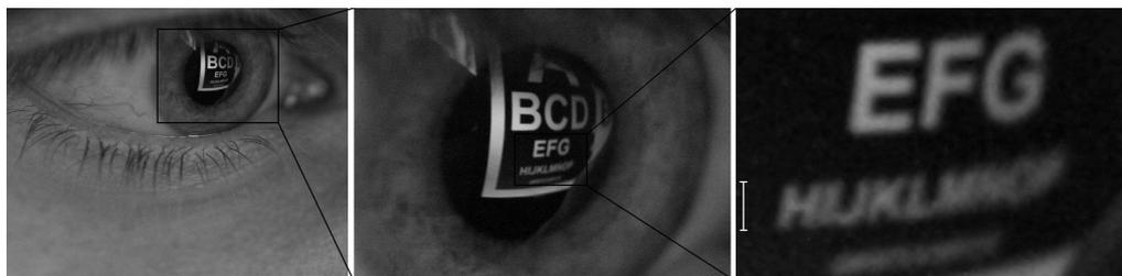
**Figure 2.3:** Image taken with a macro lens from short distance, where additionally the distance between the eye and the monitor was reduced. Readability is essentially limited by the camera resolution.
