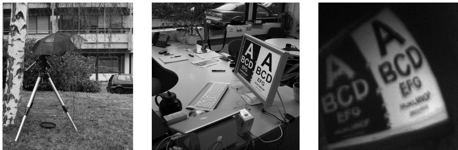
**Figure 2.21:** The attack in-field. The distance between the telescope and the office was approximately 18 meters (left), the desk where the monitor shows our test image (middle), and the captured reflections (right).
