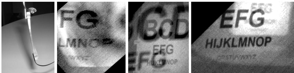
**Figure 2.17:** Reflections in eye-glasses, taken from a distance of 5 meters. Both the inner side and the outer side of glasses produce reflections. The 18 px font is readable from the reflection.
