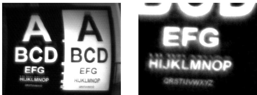
**Figure 2.2:** Reflections in a tea pot from a distance of 20 meters, using a 235 mm Schmidt-Cassegrain telescope.
