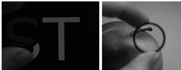
**Figure 2.34:** These images show the protection offered by an off-the-shelf optical notch filter: the letter “S” is partially covered by the filter.
