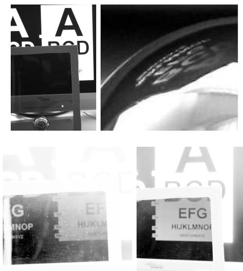
**Figure 2.32:** These images show that the protection offered by suitably aligned polarization filters is far from being perfect. While blocking most light (first image), metallic objects change polarization of light, making the monitor content readable (second image, magnification from first image). Increased exposure times still reveal the monitor contents (third image), in particular if the alignment of the two polarization filters is not perfect (fourth image).
