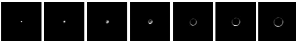
**Figure 2.24:** A sequence of measured PSFs, after stacking and post-processing. Their circular shape coined the notion of “circles of confusion” in astronomic imaging.
