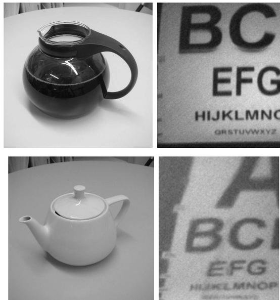
**Figure 2.16:** Reflections in two other tea pots, taken from a distance of 5 meters. The 18 px font is readable from the reflection in the top picture, and almost readable in the bottom picture.
