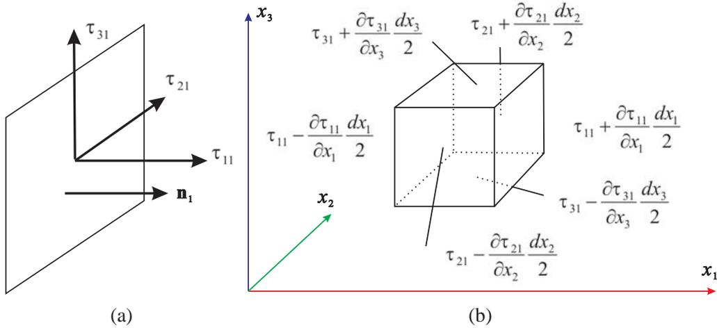
Figure 2.6: (a)Stress tensor on one surface of an element;(b) Surface stresses on an element moving with the flow, only stresses in the  $x_1$  direction are labeled.
