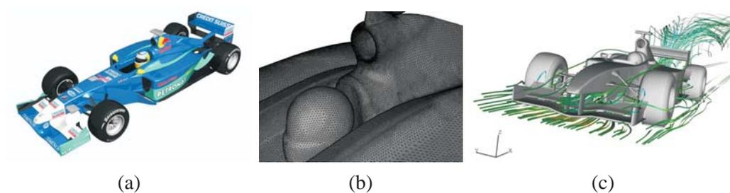
Figure 2.9: A CFD example for the Red Bull Sauber C-20 F1 racing car using CFD software *Fluent* [Flu02]: (a) A model of the car; (b) The surface mesh in the cockpit area; (c) Path lines around the vehicle.
