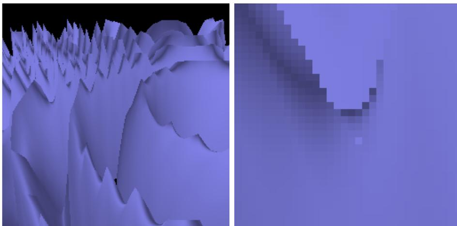
Figure 4.12: Left: The Marschner-Lobb data set approximated with a repeated linear cell intersection. Right: Close-up view reveals only subtle differences between linear and repeated linear interpolation.
