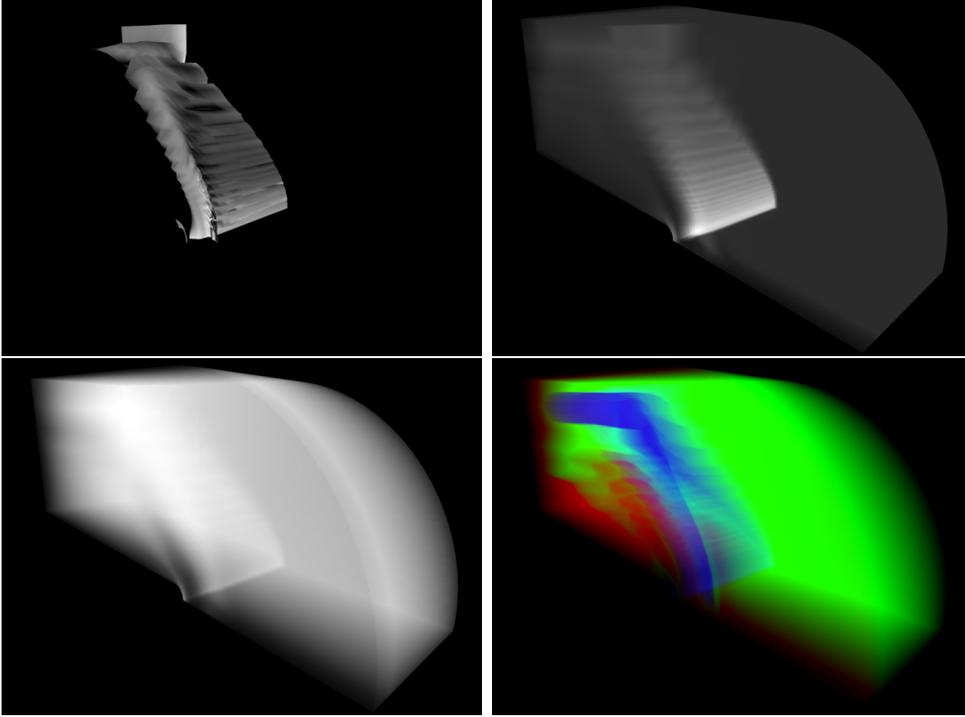
Figure 6.7: Upper Left: *The tetrahedral Blunt-fin data set rendered as an iso-surface*, Upper-right: *maximum-intensity-projection*, Lower-left: *semi-transparent rendering*, and Lower-right: *with transfer functions*.
