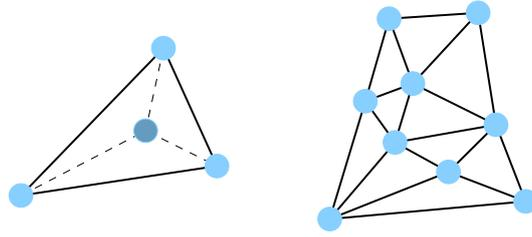
Figure 2.7: Unstructured volume data sets consist of point clouds only and therefore have no adjacency information. Since this information is needed, e.g. for interpolation, it is common to apply a Delaunay tetrahedralization [Choi02], i.e. each cell is now a tetrahedra (left) with four values. All connected tetrahedra construct a tetrahedral mesh.
