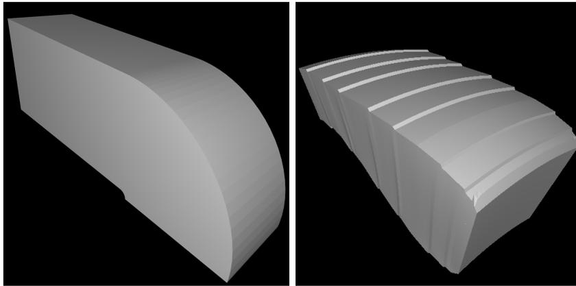
*Figure 6.3: Left: Boundary representation of the Blunt-fin data set. This is identical for the tetrahedral and hexahedral cases, since all boundary faces are decomposed into triangles. Right: Boundary representation of the Combustion Chamber consisting of hexahedral primitives. Each hexahedral boundary face is decomposed into two triangles.*
