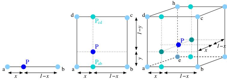
Figure 2.8: From left to right: *Linear interpolation between points a and b. Interpolating between points c and d and applying one subsequent interpolation results in a bilinear interpolation (middle image). Based on similar ideas, a tri-linear interpolation can be derived from the points a - h (right image).*
