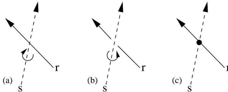
Figure 6.2: Three possible cases for the Plücker test: Looking toward the direction of  $s$ , (a) ray  $r$  passes counter-clockwise about line  $s$ , (b) ray  $r$  passes clockwise about line  $s$ , and (c) ray  $r$  intersects line  $s$ .
