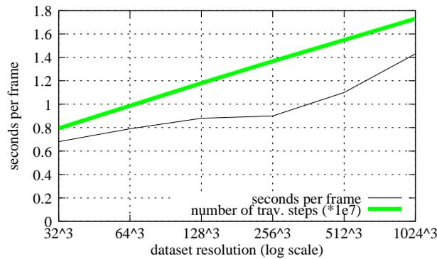
Figure 4.14: A scalability chart of the implicit kd-tree with increasing data set resolution. The resolutions of the synthetic Marschner-Lobb varies from 32<sup>3</sup> up to 1024<sup>3</sup>. This logarithmic scalability leads to a performance drop by a mere factor of 2.1 despite the fact that the data size increases by 4.5 orders of magnitude.
