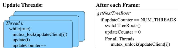
Figure 5.4: Each thread runs independently and increments a global counter, which is checked after each rendered frame. The display master unlocks the update threads for building the next kd-tree once the tree update is complete. Locking and unlocking of the counter is omitted.
