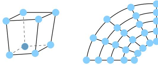
Figure 2.6: Like regular cells, curvilinear cells consist of eight neighboring values. The position of each value within a cell is arbitrary, as long as no overlapping between two cells is introduced.
