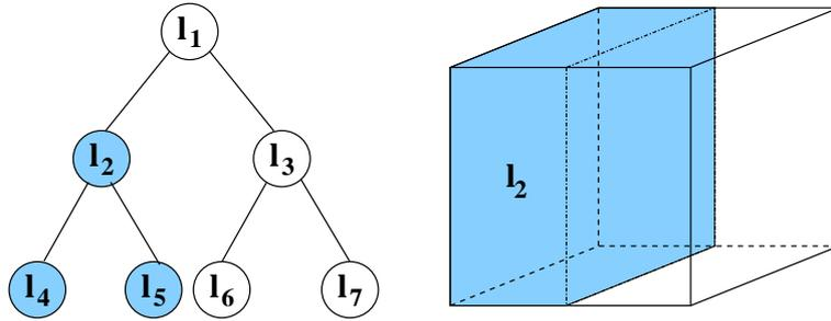
Figure 5.2: In this example, two processor cores update the complete tree. By assigning to each tree the subvolume corresponding the splitting plane, both subtrees can be independently built and merged together. At the same, a split in the middle guarantees time load balancing.
