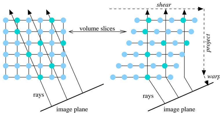
Figure 3.3: Instead of shooting rays from the view plane, the volume slices are sheared so that all rays are perpendicular to the slices, which simplifies the traversal tremendously. This sheared image must be warped in a second step allowing for a correct display of the rendered volume. For Perspective rendering, each slice needs an individual scaling factor for re-sampling.
