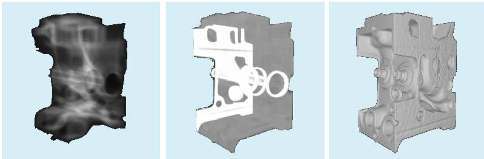
*Figure 2.9: The engine is a small data set based on regular grids with an 8 Bit scalar value. From Left to Right: Semi-transparent rendering of the density distribution, maximum intensity projection, and rendering of the iso-surface at  $\rho_{iso} = 118$ .*
