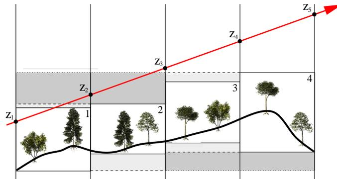
Figure 5.9: Top-level terrain kd-tree traversal. Dashed and dotted lines indicate how min/max  $z$ -values of kd-tree leaf nodes can be combined recursively to form the min/max  $z$ -values for inner nodes.
