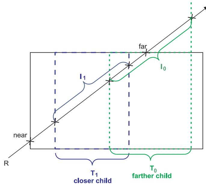
Figure 5.12: During each traversal step, the ray intersects four planes which are defined by the children bounds. This results in two (possibly overlapping) intersection intervals  $I_{\{0,1\}}$  along the ray. A child is only traversed iff its intersection interval overlaps the traversal interval defined by  $I = [near, far]$ . Examination of the closer child allows for early ray termination.
