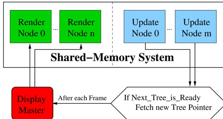
Figure 5.3: The shared-memory system is separated into render and update nodes, which do not communicate with each other since the display master controls the render and update tasks.
