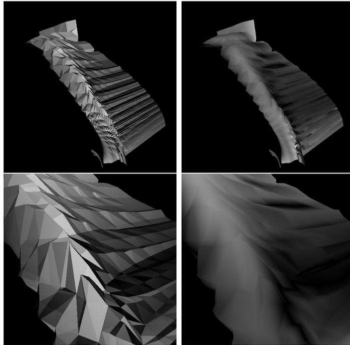
Figure 6.8: Overview (top) and close-up views (bottom) of both normal calculations. Left: Normals per tetrahedron result in severe artifacts while, Right: weighted vertex normals leads to smooth color transitions.
