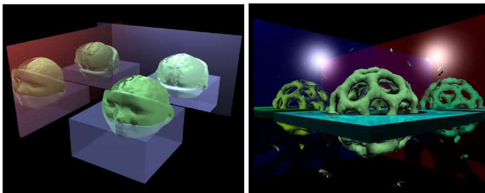
*Figure 7.1: Left: A test scene showing mixed surfaces and interactive iso-surface volume rendering with roughly 2 fps at  $640 \times 480$  resolution on a dual Intel Pentium-4 2.2 GHz system. Right: Seamless integration with surface ray tracing. The volume data set, in this case the Bucky-ball, is augmented and surrounded by reflective surfaces and light sources.*
