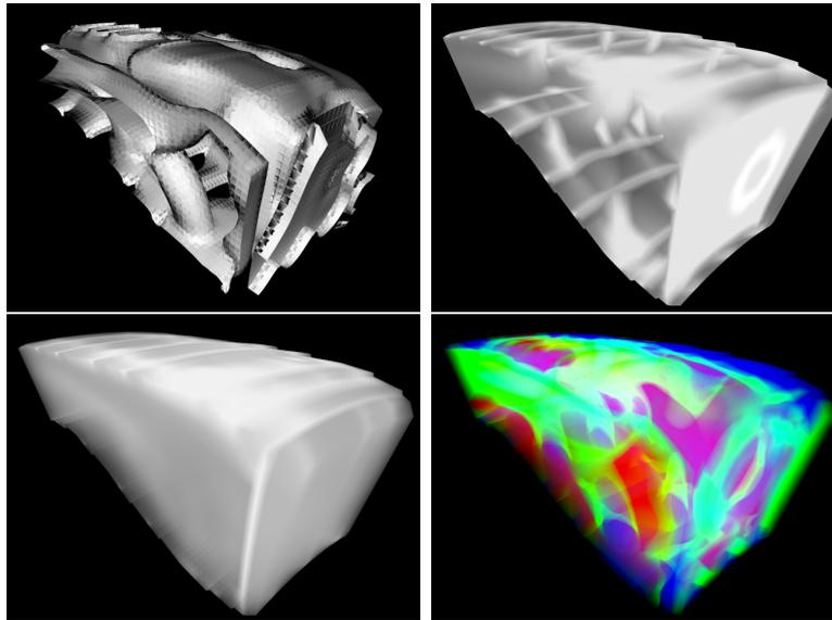
*Figure 6.15: Various renderings of the Combustion Chamber data set. Upper-left: rendered as iso-surface, upper-right: maximum intensity projection, lower-left: semi-transparent rendering, and lower-right: with transfer functions.*
