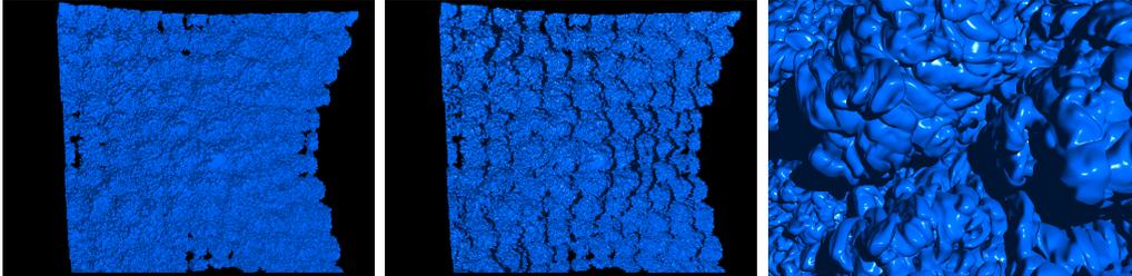
Figure 4.16: The LLNL data set, a  $2048^2 \times 1920$  simulation of a Richtmyer-Meshkov Instability. Left: Entire data set with directional light Shader. Middle: Same view, but with additional shadows. Right: Zoom-in of the surface to show the effect of shadows. Even such a complex data set of 24 GB of data can be rendered interactively on a single PC. At  $640 \times 480$  pixels, these images render at 0.9, 0.3, and 1.1 fps on a single 1.8 GHz Dual-Opteron with 6 GB RAM.
