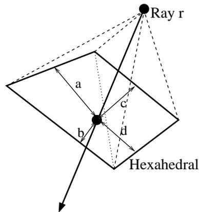
Figure 6.13: This figure illustrates why the Plücker test fails to provide meaningful parametric coordinates in the case of a hexahedral face. The scaling factor for the Plücker tests *a* and *b* differs from the one for *c* and *d*, since they were calculated using two different tetrahedral volumes.
