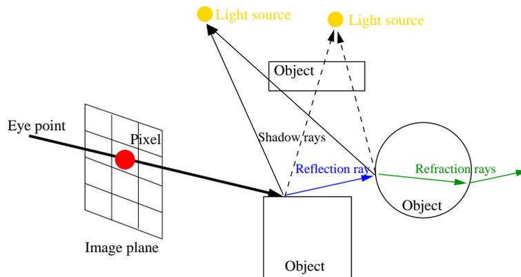
Figure 2.1: In ray tracing, rays are shot from the eye point through each pixel of the image plane. To account for shadow or material properties like reflection and refraction, secondary rays are traced recursively in the scene.
