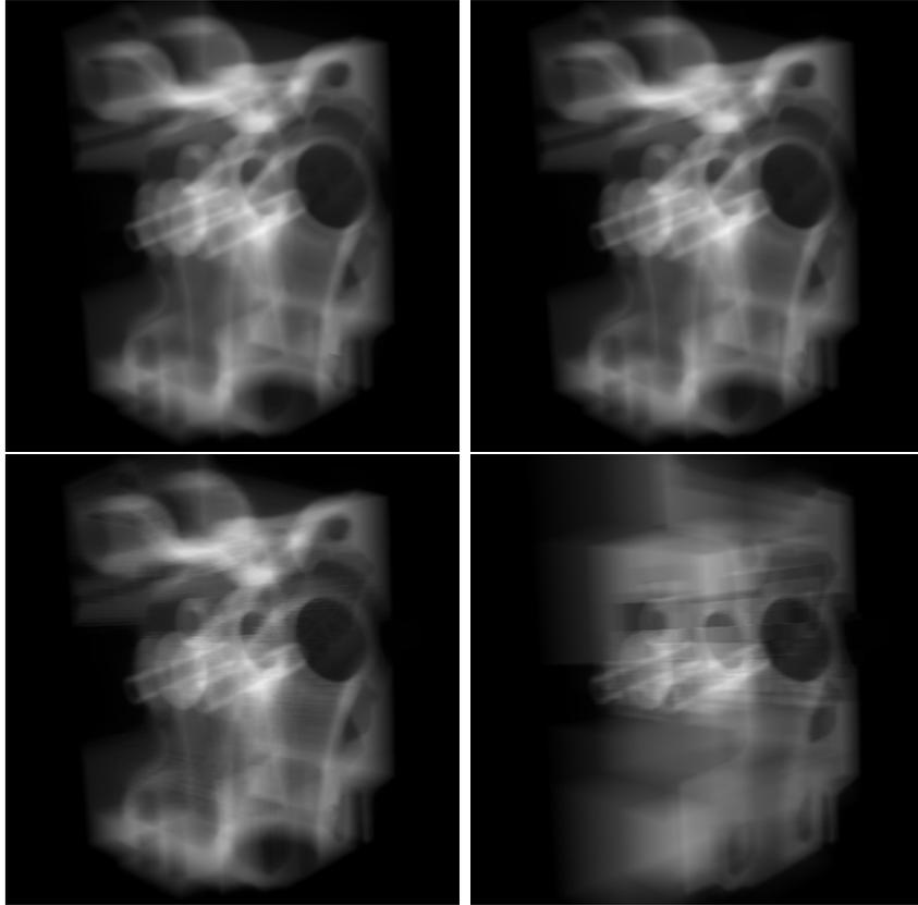
*Figure 4.19: The engine data set rendered x-ray like with no threshold (upper-left), threshold 64 (upper-right), threshold 128 (lower-left) and threshold 192 (lower-right). Note that even for a fairly high threshold, regions with low homogeneity are still clearly visible.*
