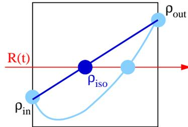
Though a bilinear interpolation for computing  $\rho_{in}$  and  $\rho_{out}$  suffices, it is generally faster to apply a trilinear interpolation since this avoids extracting the four scalar face values (which is, strictly speaking, also hardware-dependent). Another advantage is that trilinear interpolation works in favor of ray-parallel SIMD code, since it cannot be guaranteed that all rays enters and exits the cell at the same face.
