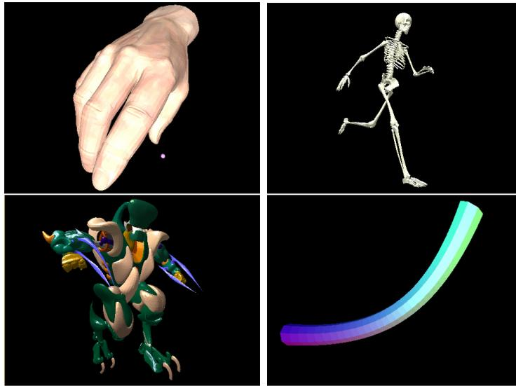
Figure 5.13: Sample images of dynamic scenes rendered in real time with 10 to 56 fps at  $512 \times 384$  screen resolution on both prototype FPGAs. Upper-left: *Hand* (17k triangles, 33 fps), upper-right: *Skeleton* (16k triangles, 34 fps), lower-left: *Helix* (78k triangles, 10.5 fps), and lower-right: *Pipe* (0.5k triangles, 56 fps).
