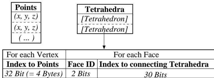
Figure 6.9: The data structure for the tetrahedral traversal algorithm consists of two tables. Table Points contains all 3D vertices. Table Tetrahedra holds entries for the Tetrahedron structure. Each Tetrahedron structure have four indices for the vertices as well as a face-id and a connection-id.
