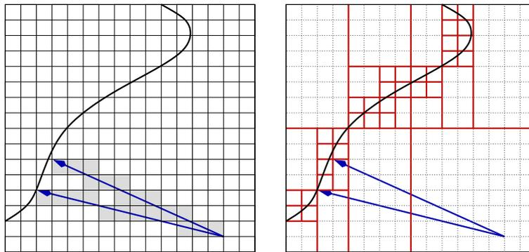
Figure 4.2: Left: Traversing all cells along the rays until an iso-surface is hit. Right: A top down traversal in a min/max hierarchy can be used to quickly skip regions without boundary cells.
