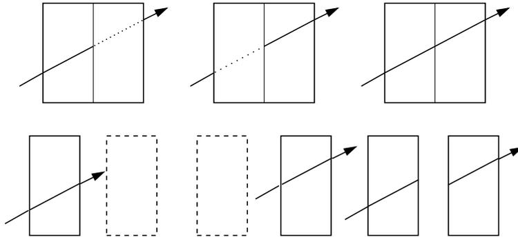
Figure 4.4: The three traversal cases are shown above. From left to right: the ray segment is in front of the splitting plane, the ray segment is behind or overlays the splitting plane. This can be easily extended when shooting four rays in parallel, e.g. using the SSE extension [Intel].
