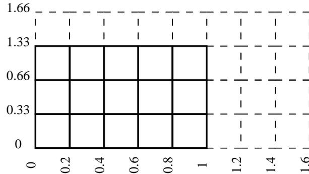
Figure 4.7: In this example, a grid consisting of  $3 \times 5$  cells is embedded in a virtual  $4 \times 8$  grid with a balanced kd-tree. By choosing appropriate split positions, it can be guaranteed that virtual cells never lie outside the scene bounds  $[0..1]^2$ , and thus will never be traversed by a ray. As a consequence, the nodes do not have to be stored and therefore consume no additional memory.
