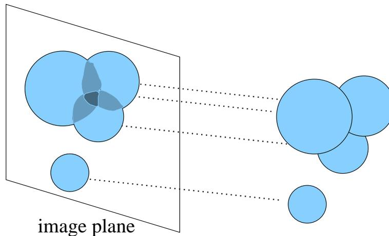
Figure 3.2: Vertex projection interprets the scalar values (illustrated here as varying point sizes) as a spatial extent (i.e. footprint) projected onto the image plane. Accumulating these footprints per pixel yields the final color.
