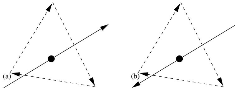
Figure 6.4: Two different configurations with the same (positive) intersection result: (a) the ray passes clockwise about all line segments of the triangle, hence all signs are positive, and (b) the ray passes about counter-clockwise all line segments, and therefore all signs are negative.
