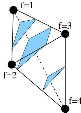
Figure 6.6: A tetrahedron with associated function values at all four vertices. Possible iso-surfaces (blue) are shown for  $f = 1.8$  (triangle),  $f = 2.5$  (quad), and  $f = 3.7$  (triangle). Values outside the range, e.g.  $f = 0$ , produce no iso-surface.
