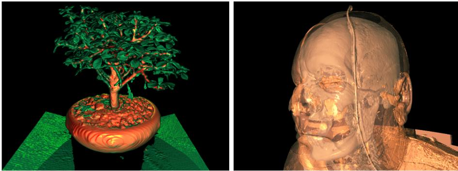
*Figure 4.3: Implicitly culling non-contributing branches of the implicit kd-tree during traversal also enables rendering of multiple iso-surfaces at the same time. Left: The bonsai tree, with a green iso-surface for the leaves, and a brown one for the trunk. Right: The Visible Female’s head, with bones visible through the semi-transparent skin surface.*
