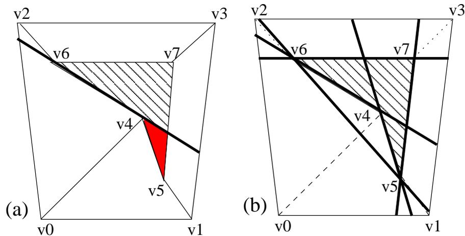
Figure 6.12: (a) The concave face illustrated cannot be handled correctly with the approach discussed previously, since it is impossible to test line  $v_4 \rightarrow v_5$  appropriately with respect to the colored area. (b) As a possible solution, the convex hull of the concave face is partitioned into triangles, which can then be handled separately. This includes two additional calculations of Plücker coordinates and a test for concave polygons.
