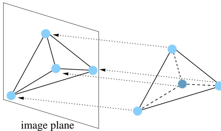
*Figure 3.1: Using projection, all primitives are projected onto the image plane before processing. In this example, a tetrahedron is projected onto the image plane resulting in the loss of depth information if the  $z$ -value is not maintained otherwise.*
