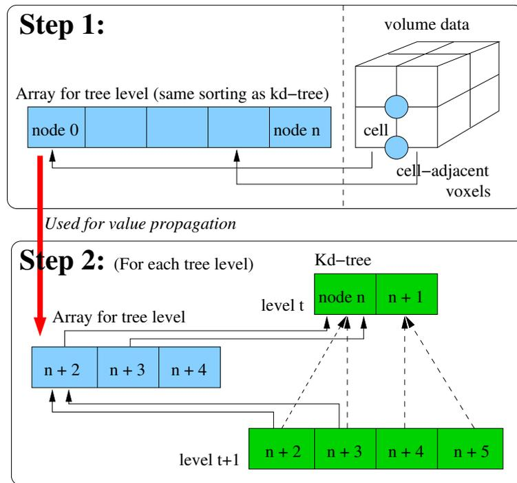
Figure 5.1: In the first step, all values are fetched sequentially from the data set and the information to be stored is sorted into the tree. The following step propagates these values bottom-up in a breadth-first manner. Since adjacent cells share four voxel, they do not have to be fetched twice, i.e. only four instead of eight values must be fetched per cell.
