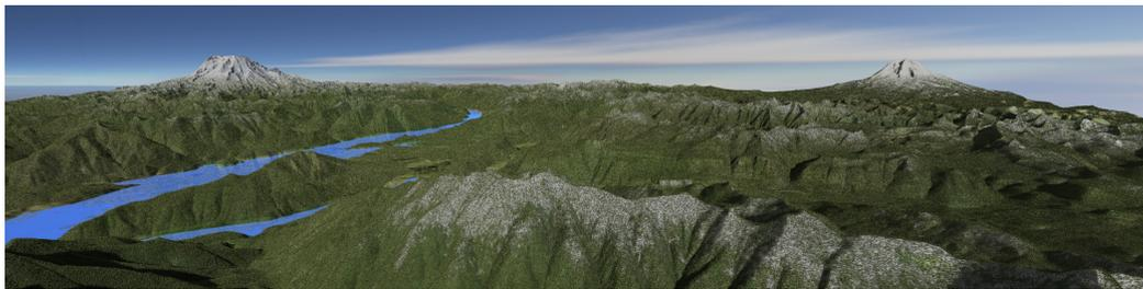
*Figure 5.7: A panoramic view over a highly complex model of the Puget Sound Area. The ground terrain consists of 134 million triangles. It is covered with billions of plant instances, where each plant model is made up of several thousand polygons.*
