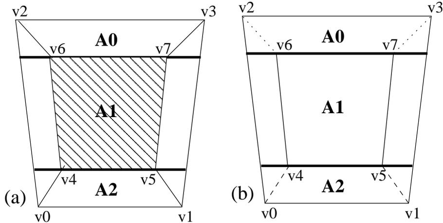
Figure 6.11: a) To determine the exiting face, the hexahedron is subdivided into three areas. (b) The next step is then to check which face is intersected by applying up to two additional Plücker tests ( $A_0$ : dotted edges,  $A_1$ : solid edges, and  $A_2$ : dashed edges).
