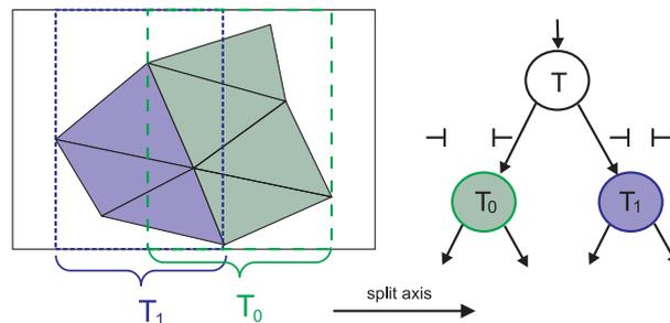
Figure 5.11: Each inner node is split into two overlapping subsets ( $T_0$  and  $T_1$  in this example). Note that only one splitting axis is stored per level. This subdivision continues until there is only one primitive per node.
