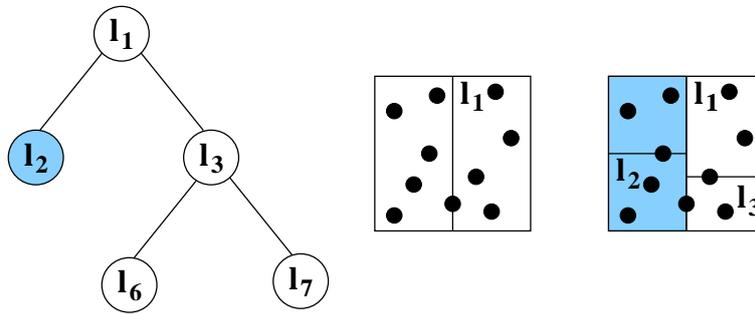
Figure 4.1: An example of a 2D kd-tree. The first split  $l_1$  separates all 2D points with respect to the  $x$ -value, while  $l_2$  and  $l_3$  separate points with respect to the  $y$ -value. In this example it is assumed, that the  $x$ -value of the searched point is greater than  $l_1$  and hence, the colored part of the point does not need to be investigated further.
