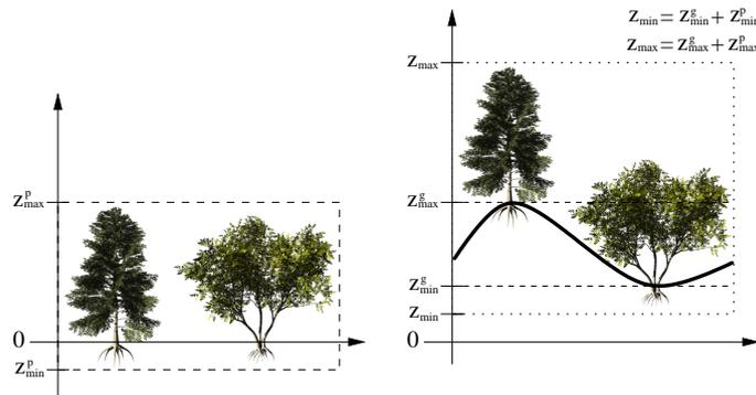
Figure 5.10: Approximate calculation of the min/max  $z$ -values of terrain bounding boxes. Left: Bounding box of a plant sub-scene. Right: The ground bounding box extended by the sub-scene bounding box.
