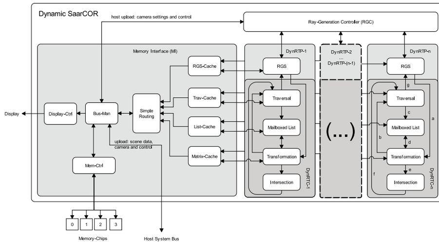
Figure 7.3: Data paths of a generic variant of a fixed function SaarCOR architecture for dynamic scenes. The SaarCOR prototype implements this architecture but uses only a single pipeline and has no cache for shading data. A fairly detailed description of the prototype can be found in Section 7.3.
