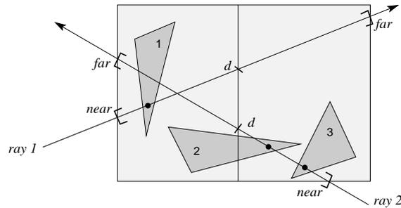
Figure 2.19: This example illustrates why termination of a ray may not be checked right after popping from stack but only after a voxel has been intersected using a valid state. The left child is entered first and the invalid ray 2 has a hit-point with triangle 2. When the right child is popped ray 2 becomes valid and the hit-point on triangle 2 becomes a valid criterion for early termination. If ray termination is checked before the right voxel was intersected triangle 3 will be missed.
