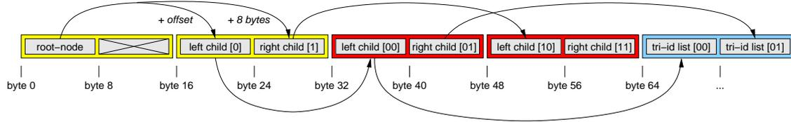
Figure 2.11: Memory layout of the left-most kd-tree in Figure 2.4
