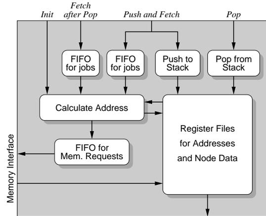
Figure 4.8: Data paths of the traversal memory interface which manages the stack for node addresses and performs memory requests for node data.
