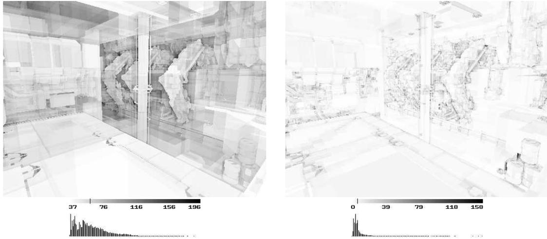
Figure 2.23: Cost images of a good kd-tree with low cost for traversal (left image) and intersections (right image). The darker a pixel is colored the more operations had to be performed to compute it. The histograms give an overview of the distribution of costs (measured in number of operations) while the bar on the scale marks the average workload.
