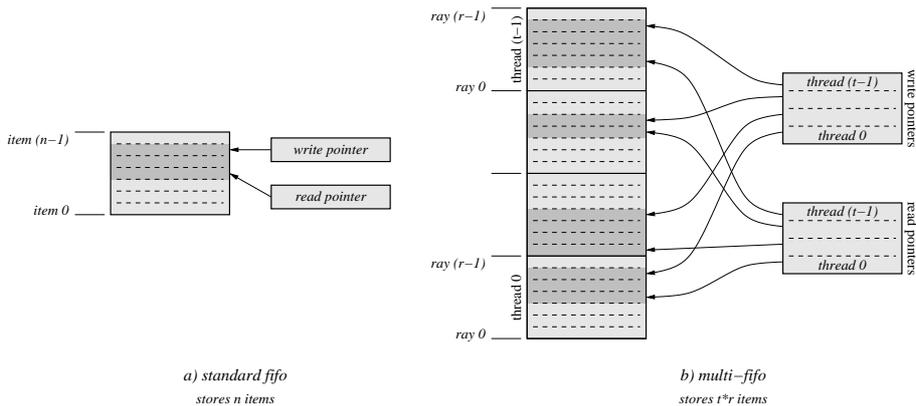
Figure C.1: A standard FIFO for  $n$  elements and a multi-FIFO which can store  $t \times r$  elements. An implementation of these FIFOs which can insert and deliver an item in every cycle requires dual-port registers and register files for reading and writing in the same cycle. The blocks marked in grey are continuous regions of memory which shows the simplicity of this design.
