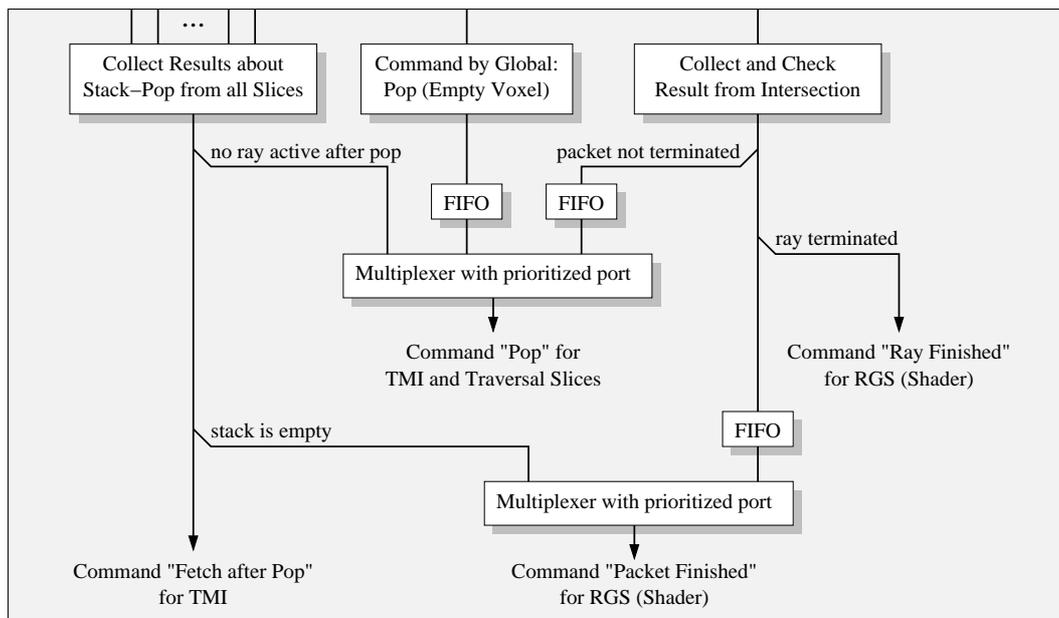
Figure 4.7: Control flow of Collect Hits. It can be seen that the most interesting component is only a simple management for several sources that can issue the same command simultaneously.
