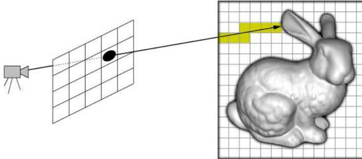
Figure 2.3: Example for traversal of a static scene using a regular grid.
