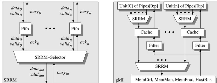
Figure 6.2: Data paths of the *simple round-robin multiplexing* (SRRM) interconnection scheme and a general version of the memory interface (gMI). Here the simple point-to-point connection scheme and the shared caches are clearly visible.
