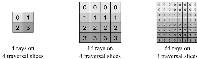
Figure 8.3: Assignment of rays to traversal slices using the sub-optimal method  $C^*$  which is almost identical to method  $C$  presented in Chapter 4.2.1. Here for packets with  $2^n$  rays, a ray with packet-coordinates  $(x, y)$ , with  $0 \leq x, y < n$  is assigned to traversal slice  $t = \frac{x+y \cdot n}{\text{number of slices}}$ .
