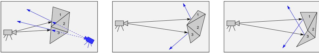
Figure 2.17: Tracing reflection rays splits into three cases (from left to right): the trivial case of a planar mirror which yields the same rays as if the camera would have been mirrored on the planar surface, reflections on strictly convex surfaces also do not lead to any problems (except for cases with numerical instabilities), but concave objects can cause rays that cross, which might lead to errors.
