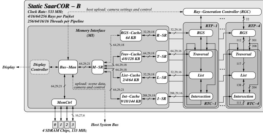
Figure 8.6: Data paths of Static SaarCOR Variant B. Functional units shown in white are simulated using a cycle accurate model while grey boxes (the Display Controller and the SDRAM chips) use a behavioral model only.
