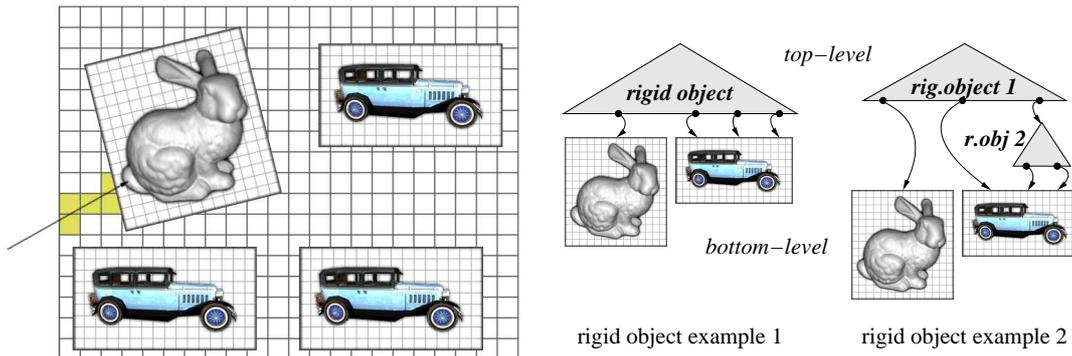
Figure 2.13: Example for traversal of a dynamic scene using rigid objects. On the left the execution of the traversal algorithm is illustrated while on the right there are two examples for the hierarchical structure of the scene. In the second example two cars are grouped together in a rigid object allowing for simultaneous movements. On any change of a rigid object (either its triangles or its transformation matrix) the kd-trees of all rigid objects above them have to be recomputed.
