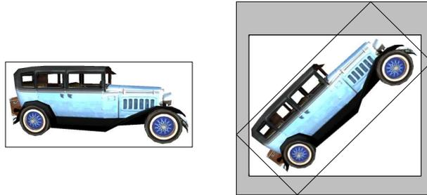
Figure 2.14: Example for an rigid object with its axis-aligned bounding box and the same object and its bounding boxes rotated by 45 degrees. It shows that the axis-aligned bounding box of the rotated object is much larger (the grey part) than required.
