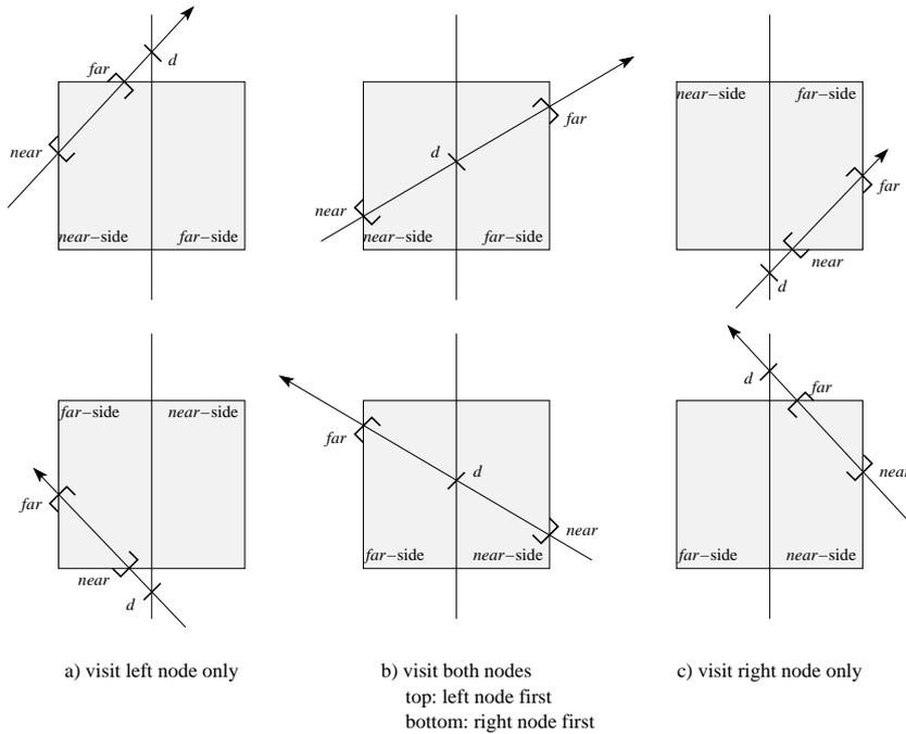
Figure 2.6: The six different case of kd-tree traversal.
