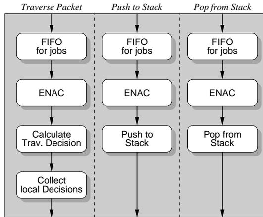
Figure 4.5: Data paths of a traversal slice with its three functional units. Each unit is implemented as a simple static pipeline without conditionals or loops.
