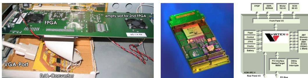
Figure 7.8: The left image shows the inside of the PC which is equipped with the prototyping board. Each PCI-board can hold up to two mezzanine cards (the image in the middle) containing an FPGA, 6 banks of SRAM and (optionally) DDR-RAM. The right image shows the data paths of this card. Additionally, the left image shows the self-made DA-converter interfacing the prototyping board to a standard VGA-monitor. (Both images on the right are courtesy of Alpha-Data [Alp03].)
