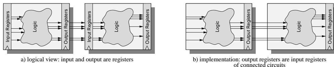
Figure 7.1: The inputs and outputs of each black box come from registers. The implementation uses only output registers and therefore input registers are only pointers to output registers (image b). However, wire delay between boxes can be simulated by increasing the delay of the corresponding black box.
