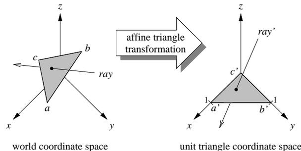
Figure 4.10: The unit triangle intersection method consists of two stages: First the ray is transformed, using a triangle specific affine triangle transformation. In the second stage, a simple intersection test of the transformed ray with the unit triangle is performed.
