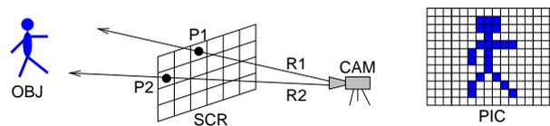
Figure 2.1: Basic Principle of Ray Tracing
