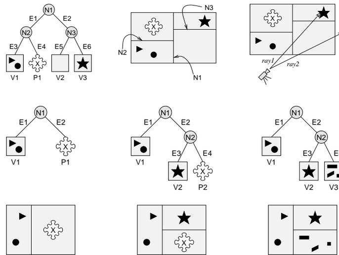
Figure 6.4: The first row shows an example of a kd-tree with a placeholder object P1. This object can be a voxel containing a few triangles as imposters. When rendering the view depicted in the right most image the placeholder object is not touched and thus does not need to be replaced. In the second row it is shown how placeholder objects are replaced recursively from one frame to the next frame.
