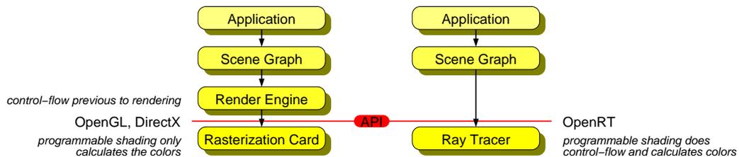
Figure 1.3: Structure of rasterization and ray tracing applications.
