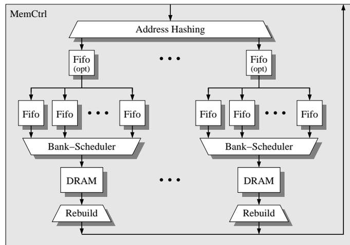
Figure 6.3: Data paths of the memory controller that allows for performing random memory accesses at a bandwidth close to the theoretical maximum. It utilizes for each internal memory bank a small FIFO and optionally an additional FIFO for each DRAM to further decouple the banks. Each word is fetched sequentially from memory using burst transactions from a single memory chip and then the unit *rebuild* arranges the final data word.
