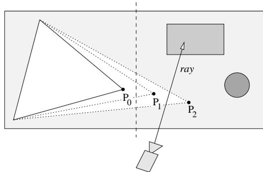
Figure 6.5: The geometry processor can modify any geometric primitive when fetched from memory. In the example above the vertex  $P_i$  of the triangle moves depending on the current time between position 0 and 2. However, since the kd-tree is independent of the time both voxels must contain a reference to the triangle to avoid missing an intersection (e.g. when the vertex is at  $P_2$  and the right voxel would not contain the reference to the triangle).
