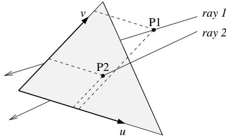
Figure 2.10: Examples for ray-triangle intersection tests using the barycentric coordinates of the position where the ray pierces the plane spanned by the triangle. The ray *hits* the triangle if for the coordinates  $(u, v)$  it holds  $0 \leq u, v \leq 1$  and  $(u + v) \leq 1$  as can be seen for ray 2. Ray 1 *misses* the triangle since P1 has  $(u + v) > 1$ .
