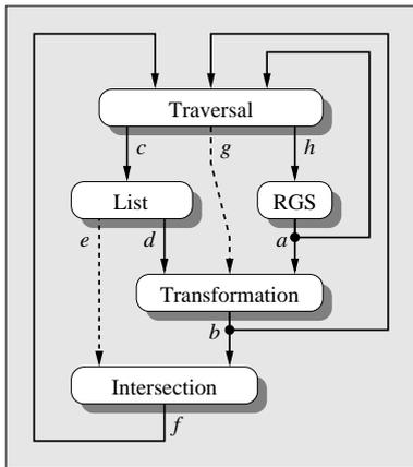
Figure 4.2: Unoptimized data paths for ray data and control flow. The stacks in the traversal slices of the traversal unit and in the transformation unit are not shown for the sake of simplicity.
