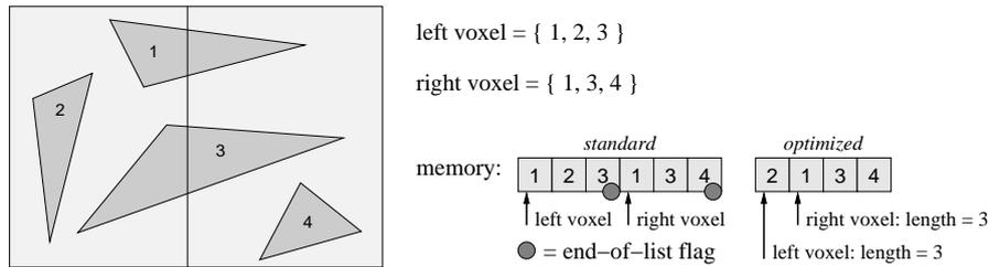
Figure 4.9: Example for optimized storage of triangle-ID lists. With an end-of-list flag only the standard variant of storing lists of IDs can be used. With an additional adder the optimized variant of storing *packed lists* of IDs can be used which allows for great savings in memory storage.
