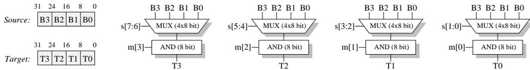
Figure 5.4: Implementation of the swizzle instruction on a SCPU with 32 bit wide registers. The content of the second source register is used as parameters to specify which bytes to select (using  $s[7:0]$ ) and which bytes to mask (using  $m[3:0]$ ).
