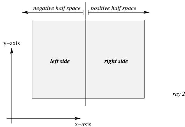
Figure 2.5: Simplified labels for kd-trees shown in examples: all splitting planes are drawn parallel to the y-axis independent on their actual orientation and the *negative half space* formed by the splitting plane is labeled as being *left of the splitting plane*.
