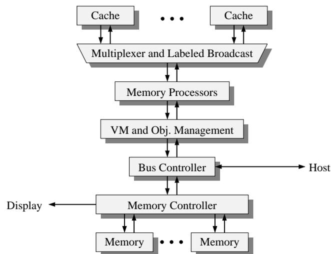
Figure 6.1: Data paths of the memory interface. All units of the same type (e.g. traversal units from all pipelines) share the connection to an *item-based cache* using a simple round-robin multiplexed bus for requests and a labeled broadcast for data sent by the memory.
