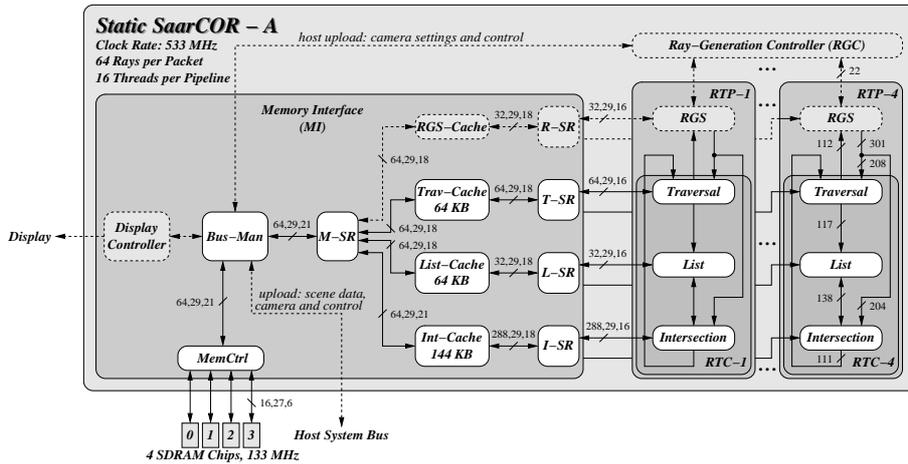
Figure 8.2: Data paths of Static SaarCOR Variant-A. Functional units shown in white are simulated using a cycle accurate model while grey boxes use a behavioral model only.
