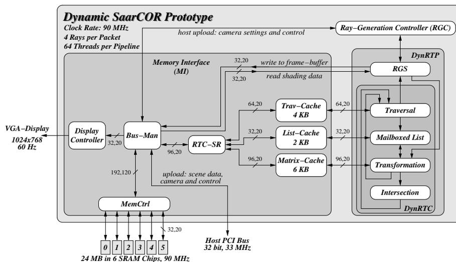
Figure 8.9: Data paths of Dynamic SaarCOR Prototype. In contrast to the *static SaarCOR* variants, the list unit implements mailboxing to avoid multiple intersection of objects and triangles.
