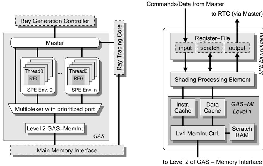
Figure 5.1: Data paths of the *general architecture for shading* (GAS) and a suitable embedding of an arbitrary *shading processing element* (SPE). The GAS provides the infrastructure to manage memory accesses, transfers ray data, starts jobs on the processing elements, and collects their results. The GAS together with the SPEs provide the functions to generate and shade rays and thus form the RGS.
