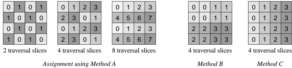
Figure 4.3: Examples of assigning a packet of 16 rays to slices. Each box denotes a pixel in screen-space with its corresponding ray(s) and the number in the box specifies the slice this pixel is assigned to.
