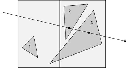
Figure 2.9: Example for traversing a kd-tree that shows the necessity to check whether a hit-point is in the current voxel: In the first step the left voxel is intersected yielding a hit-point on triangle 3. Since this hit-point is not inside the intersected voxel traversal continues with the voxel on the right leading to a valid and correctly identified final hit-point with triangle 2.
