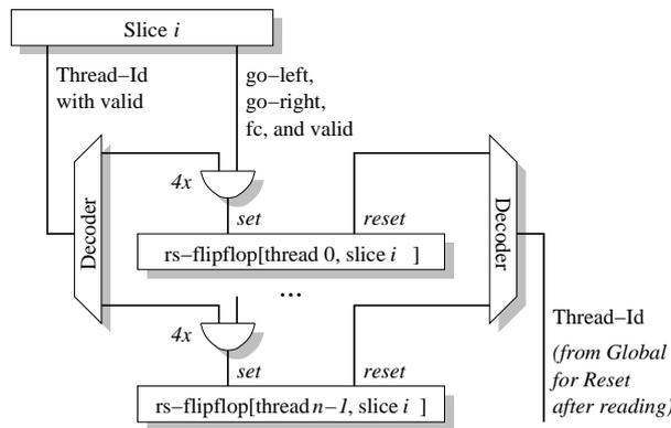
Figure C.3: Diagram of the communication between Global and the Traversal Slices.
