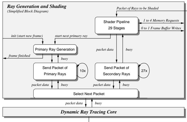
Figure 7.6: Simplified block diagram of the ray generation and shading unit.
