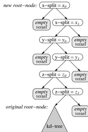
Figure 2.8: Clipping of a ray to the axis-aligned bounding box  $((x_0, y_0, z_0), (x_1, y_1, z_1))$  of a scene by putting six additional nodes on top of the scene's original kd-tree.
