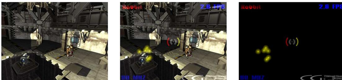
Figure 7.7: Without any special effects the left image looks rather simple. However, much nicer presentations are possible by using 2D overlay effects (the image in the middle). For comparison the image on the right shows only the overlay. (All images are rendered in  $1024 \times 768$ .)
