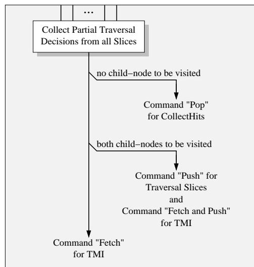
Figure 4.6: Control flow of Global. The tricky part of collecting partial traversal decisions computed out-of-order is greatly simplified as this is mostly done directly in the corresponding traversal slice. This way in Global there is no read-modify-write processing but only storing of the partial result sent by each traversal slice and therefore Global is easy to implement.
