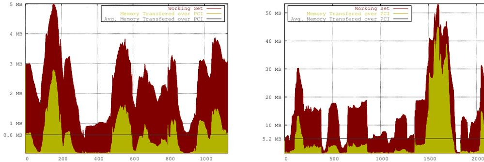
Figure 8.8: Results of the first simulation step for the *pQuake3* scene (left, with textures and light) using 8 MB card memory and the cruiser scene (right, with textures and light) with 64 MB. For each frame of the sequence it plots the size of the working set and the amount of memory transferred.
