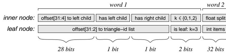
Figure 2.12: Unified data structure of the kd-tree nodes (inner nodes and leaves).
