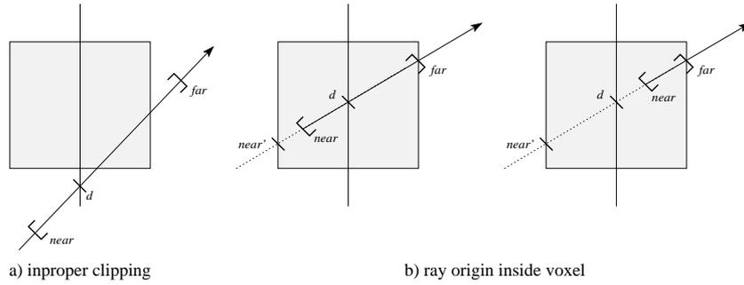
Figure 2.7: Two special cases of kd-tree traversal: a) traversal step with incorrectly set *near* and *far* values, b) a ray starting inside a voxel. All cases can be handled trivially by correctly initializing *near* and *far* to the bounding box of the scene and at the same time rejecting any updates on *near* if  $d < near$ . Inproper handling of these cases does not cause any errors but may lead to unnecessary traversal steps.
