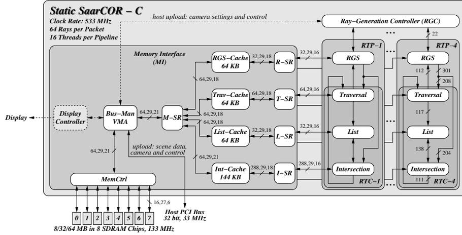
Figure 8.7: Data paths of Static SaarCOR Variant C+D. Functional units shown in white are simulated using a cycle accurate model while grey boxes use a behavioral model only.
