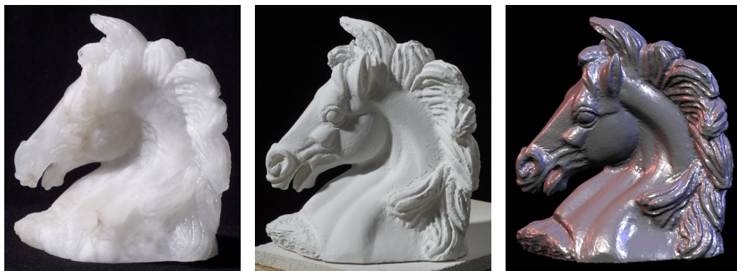
Figure 3.2: The alabaster horse. Left and middle: Photographs of the sculpture with and without subsurface scattering under identical illumination conditions. The sculpture was covered with fine dust to “turn off” subsurface scattering. Much surface detail is masked by the translucency and active optical range scanning systems have grave problems to scan the translucent object. Right: Rendering of the acquired geometry model (100 k triangles) with flat shading.
