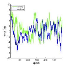
**Figure 3.13**: Positioning errors of the pedestrian positioning experiment as reported in [Peng et al., 2011]
