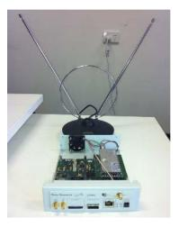
**Figure 3.7**: The sensor equipment used for FM-radio-based positioning ([Moghtadaiee et al., 2011]).
