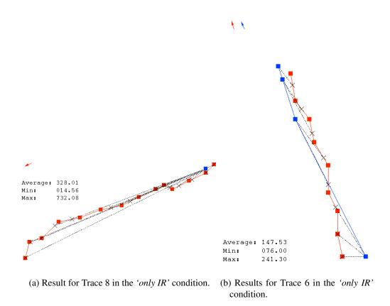
**Figure 4.35**: The worst (a) and best (b) result for the '*only IR*' condition. In Trace 8 only one IR beacon was detected. Trace 6 contains 4 detected IR beacons.
