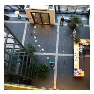
**Figure 4.31**: Traces were laid out on the floor and followed while carrying a mobile device running LORIOT.
