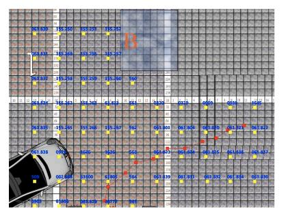
Figure 4.30: 58 active RFID tags were distributed in the DFKI foyer.
