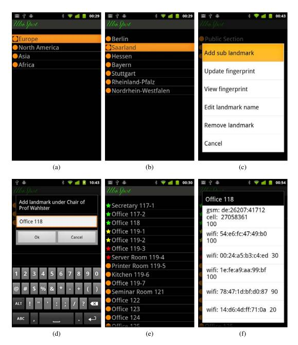
**Figure 4.14**: Training of a new location in UBISPOT: A user browses through the imported UBISEARTH location model and refines it by a new location. This location is stored with the current fingerprint.
