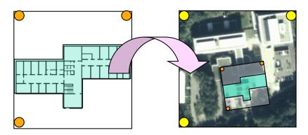
**Figure 4.10**: YAMAMOTO allows to geo-reference a model by rescaling, resizing and placing it into an already geo-referenced areal photography.
