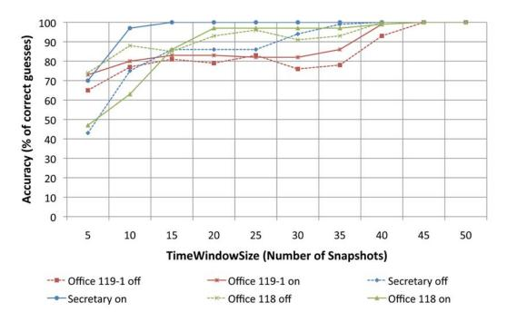
Figure 4.21: Accuracy plotted against *TimeWindowSize* when only three landmarks are stored in the trained database.
