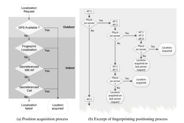
**Figure 3.12**: Flowcharts of LOCATEME's position acquisition and fingerprinting process ([Pereira et al., 2011a]).
