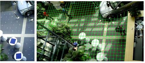
(a) Adhesive tape was used to enhance the visibility of the tile seams.
