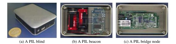
**Figure 3.9**: The WSN in the Hecht museum consists of blinds (a), stationary beacons (b) and bridge nodes (c) ([Dim et al., 2011])
