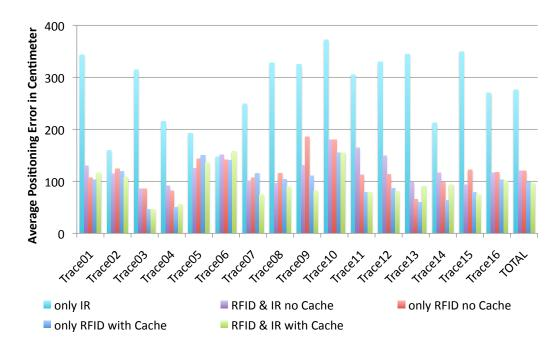
**Figure 4.34**: The average positioning error of all traces with original velocities and with respect to the five tested conditions.
