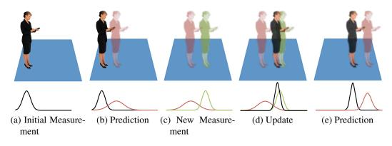
Figure 2.19: Example of a Kalman filter for positioning.
