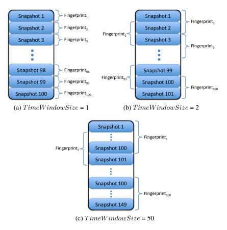
Figure 4.17: The calculation of 100 FOA fingerprints with different TimeWindowSize. Since the fingerprints are calculated by using a FIFO, 99 + TimeWindowSize snapshots are needed.
