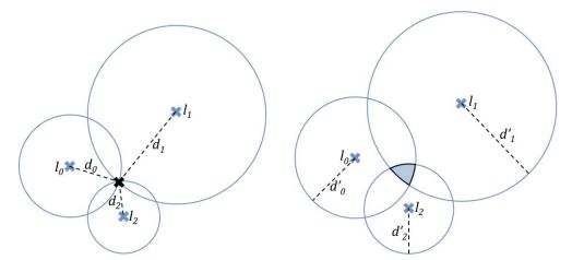
(a) Trilateration with accurate measurements (b) Trilateration with inaccurate measurements
