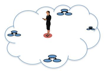
**Figure 4.6**: A cloud of geoDBNs arises around the user. Each geoDBN has a weight (indicated by the size of each geoDBN in this picture), determined by its belief that the user is standing at its position. The user's position is estimated by calculating the center of mass of the cloud.
