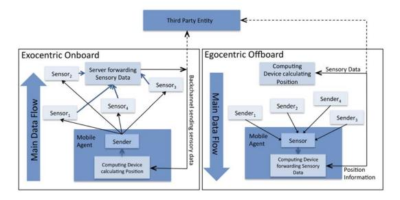
**Figure 2.9**: Onboard exocentric and offboard egocentric positioning. Sensory data is sent from the environment to the agent or from the agent to a computing device in the environment.
