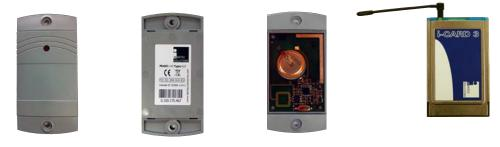
(a) Active RFID tag (b) Active RFID tag (c) Active RFID tag (d) Active RFID reader card front back circuit
