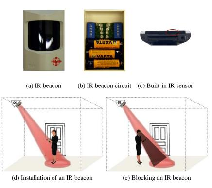
**Figure 4.23**: IR beacon as manufactured by Eyeled (a). Each beacon sends out a 16-bit wide ID, which can be configured by DIP switches. The circuit is powered by 3 AA batteries (b). The beacons can be detected and identified by standard IR sensors, which are often already integrated into mobile devices (c). IR beacons are perfect to signal points of interests (d).
