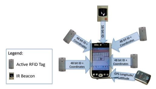
**Figure 4.22**: LORIOT uses active RFID tags and infrared beacons, which are distributed into the environment, to estimate the current position of a Windows Mobile PDA.
