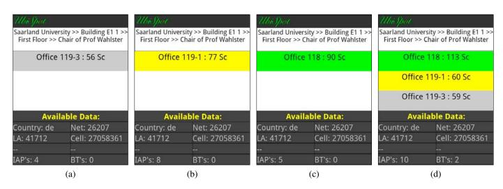
**Figure 4.15**: Output of the UI of UBISPOT: The confidence level of the system is color-coded: green for highest confidence, yellow for middle and gray for lowest confidence.
