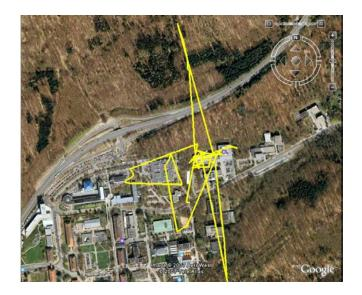
**Figure 1.1**: Positions determined over a course of 25 minutes by a GPS receiver resting on a windowsill inside building E11 on campus of Saarland University.
