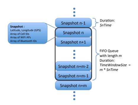
**Figure 4.3**: Calculation of Frequency-of-Appearance fingerprints with a FIFO queue of length *m* and resulting duration *TimeWindowSize*.
