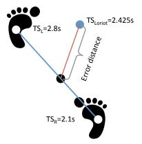
**Figure 4.32**: Ground truth time-stamps of single footsteps and LORIOT time-stamps of user positions do not necessarily coincide.
