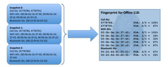
Figure 4.2: Example calculation of a Frequency-of-Appearance fingerprint with m = 3: The appearance of each ID in all three snapshots is counted out and the relative appearance is stored in the fingerprint along with a semantic description of the current position.
