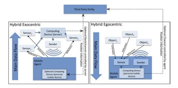
**Figure 2.8**: Hybrid exocentric and egocentric positioning. Sender and sensor are both installed either in the environment or at the agent.
