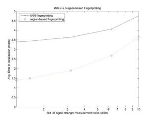
Figure 3.14: Average positioning error as shown in [Xiao et al., 2011].
