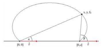
**Figure 2.15**: An iso-Doppler contour results from the measurement of one FDOA measurement ([Vesely, 2010]).
