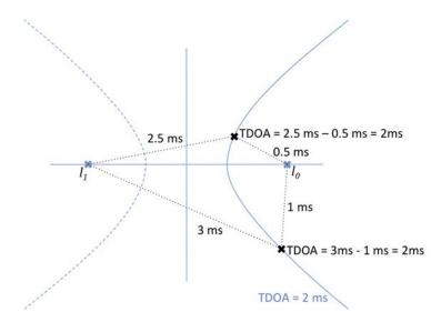
**Figure 2.14**: A single TDOA measurement results in a hyperbola with two known locations as focus points. Only one branch of the hyperbola has to be considered (marked with a solid line).
