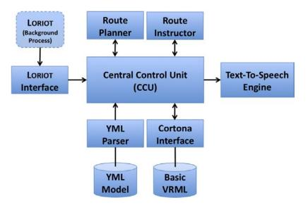
**Figure 5.2**: Components of PARKNAVI. The current user position is read from LO-RIOT to update route instructions accordingly [Gholamsaghaee, 2007].
