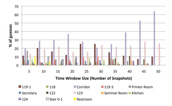
**Figure 4.19**: Hits and misses for office 119-1 not considering Bluetooth devices. Most of the time UBISPOT mistakes the office 119-1 for the corridor.
