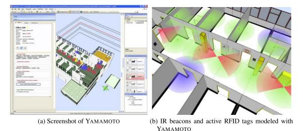
**Figure 4.9**: YAMAMOTO can be used to model a building and plan the positioning infrastructure. Shown are IR beacons (red), active RFID tags (green) and Bluetooth beacons (blue).
