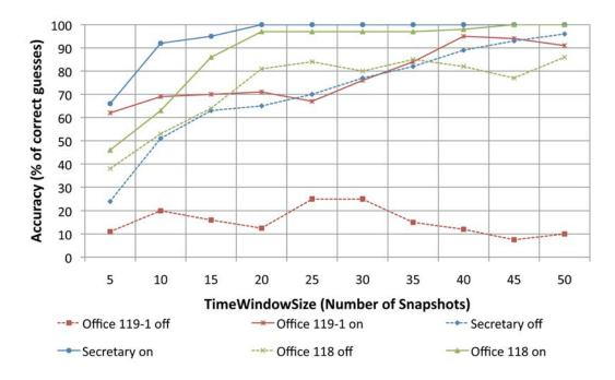
**Figure 4.18**: Recognition accuracy versus *TimeWindowSize* for three adjacent rooms. Solid lines indicate results including all available sensor data, dashed lines indicate the results when Bluetooth is not considered for the position calculation.
