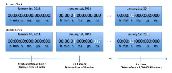
Figure 2.13: Inaccuracies of a quartz timer in comparison to an atomic clock.
