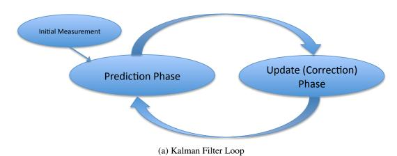
**Figure 2.18**: The Kalman filter loop: after an initial measurement, prediction phase and update phase will be repeatedly executed.
