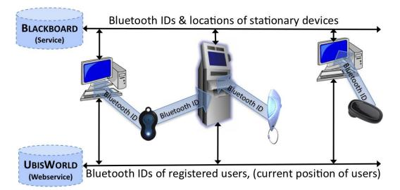
**Figure 4.12**: OUT OF THE BLUE consists of stationary devices, like desktop PCs, public displays or kiosk systems that scan their environment for mobile Bluetooth devices, like cell phones, wireless headsets or Bluetooth tags. Information can be shared via a blackboard service and registered users can store their Bluetooth IDs in UBISWORLD.
