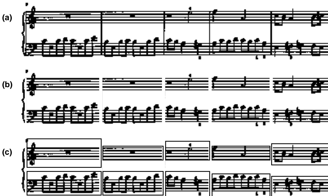
Fig.6: Accolade: (a) raw data, (b) barline removal, (c) resulting barunits
