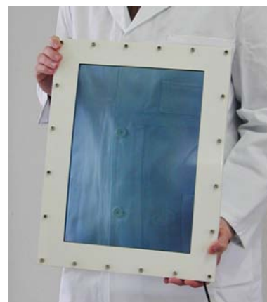
Fig. 8: Curved blue colored EC window of the INM (size 400 mm x 300 mm, curve radius 2000 mm). The transmission in the visible range (TL value, DIN EN 410) can be varied from 70 % (bleached) to 25 % (blue colored, voltage < 3 V, switching time 2-3 min).
