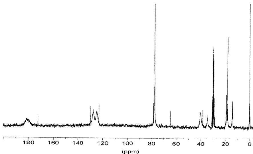
Figure 3  $^{13}\text{C}$ -NMR spectrum of hydrolysis of  $[\text{Ti}(\text{OBu}^n)_3(\text{PA})]_n$ .
