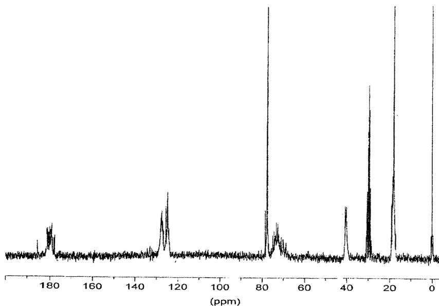
Figure 1  $^{13}\text{C}$ -NMR spectrum of  $[\text{Ti}(\text{OEt})_3(\text{PA})]_n$ .
