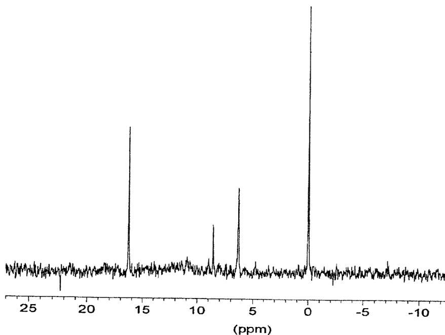
Figure 4  $^{29}\text{Si}$ -NMR spectrum of  $([\text{Ti}(\text{OBu}^n)_3(\text{PA})]_n + \text{TRES})$ .
