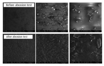
Figure 6: Scanning electron micrographs on the Taber track before and after abrasion test for polyurethane nanocomposite system PU A9, scale bars (left to right): 50 µm, 10 µm, 2 µm
