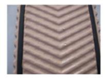
Figure 10: Heat exchanger plates coated with nanocomposite anti-adhesive systems after 4 h test in the heat exchanger at LUFA Norwest, left: epoxy nanocomposite EP A2, right: polyurethane nanocomposite PU A10
