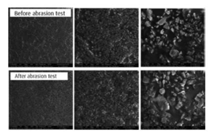
Figure 5: Scanning electron micrographs on the Taber track before and after abrasion test for epoxy-based nanocomposite system EP A1, scale bars (left to right):  $50 \mu m$ ,  $10 \mu m$ ,  $2 \mu m$
