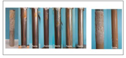
Figure 9: Cleaning behaviour of whey protein deposits in NaOH flow: stainless steel (left) and polyurethane nanocomposite coating PU A9 (right)
