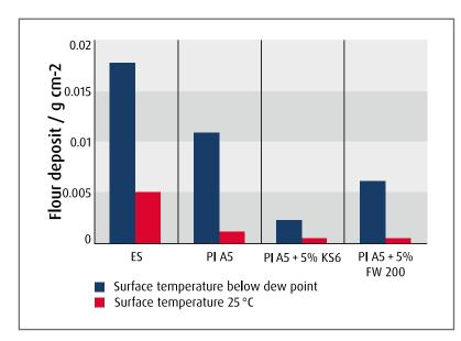
Figure 11: Gravimetric determination of flour (type 405) adhering to 1 m long stainless steel test tubes with 120 mm diameter at ambient temperature and below the dew point; ES: uncoated stainless steel, PI A5, PI A5 + carbon black FW 200, PI A5 + graphite KS6
