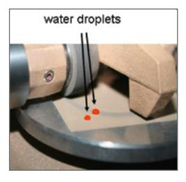
Figure 4: Direct comparison of shape of water droplet on unloaded coating surface and mechanically stressed surface (EP A1) shows that low wetting is retained after mechanical abrasion
