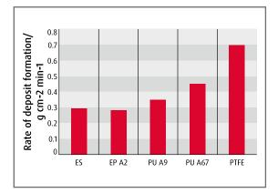
Figure 8: Deposition rates of whey proteins (10 % solution) on internally heated tubes in a flow channel, tube surface temperature 134 °C
