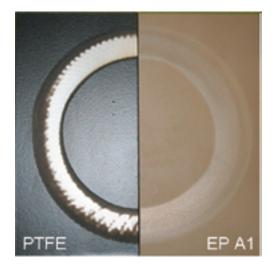
Figure 3: Result of the "Taber Abraser" test on PTFE and nanocomposite coated stainless steel after 1000 cycles
