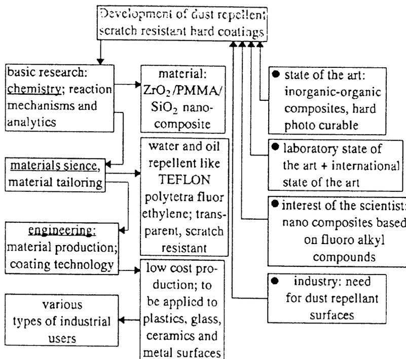
Fig. 2: Development of a dust repellent coating based on an inorganic-organic nanocomposite [after 1 - 3].
