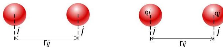
**FIGURE 2.2** Schematic representations of the non-bonded interactions. (a) Lennard-Jones potential and (b) Coulomb potential.
