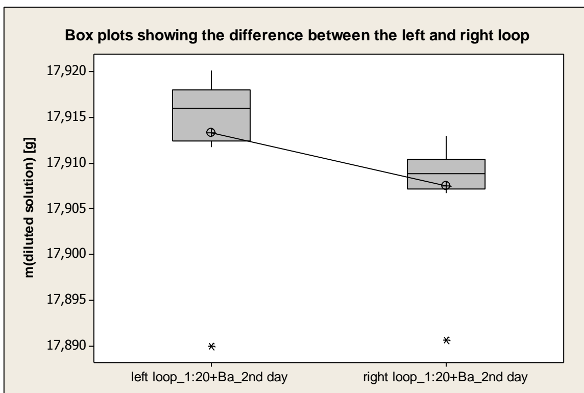
Figure 5-37: Evaluating the difference of the preparation process of the sample and QC with the help of box plots, in a 1:20 solution dilution and the addition of Ba as internal standard (second day)
