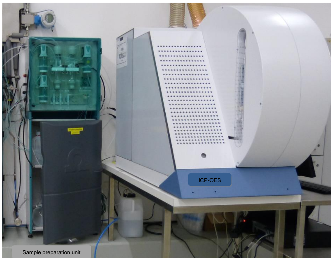
Figure 2-3: The on-line process analysis system consisting of a sample preparation unit connected to an ICP-OES
