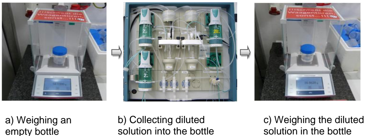
Figure 4-5: Procedure for the gravimetric determination
