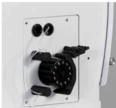
Figure 3-9: A peristaltic pump beside the spectrometer that pumps the sample and the rinsing solutions into it and waste solutions out of the device with the help of a hose system [91]
