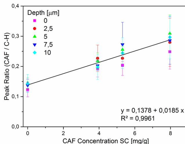
**Figure 11:** Ratio of the C-H and caffeine representing peak intensity determined by CRM as a function of caffeine concentration per mass stratum corneum determined by HPLC for five different depths with applied linear fit (mean  $\pm$  SD,  $n = 9$ ). Reproduced with permission from (66).
