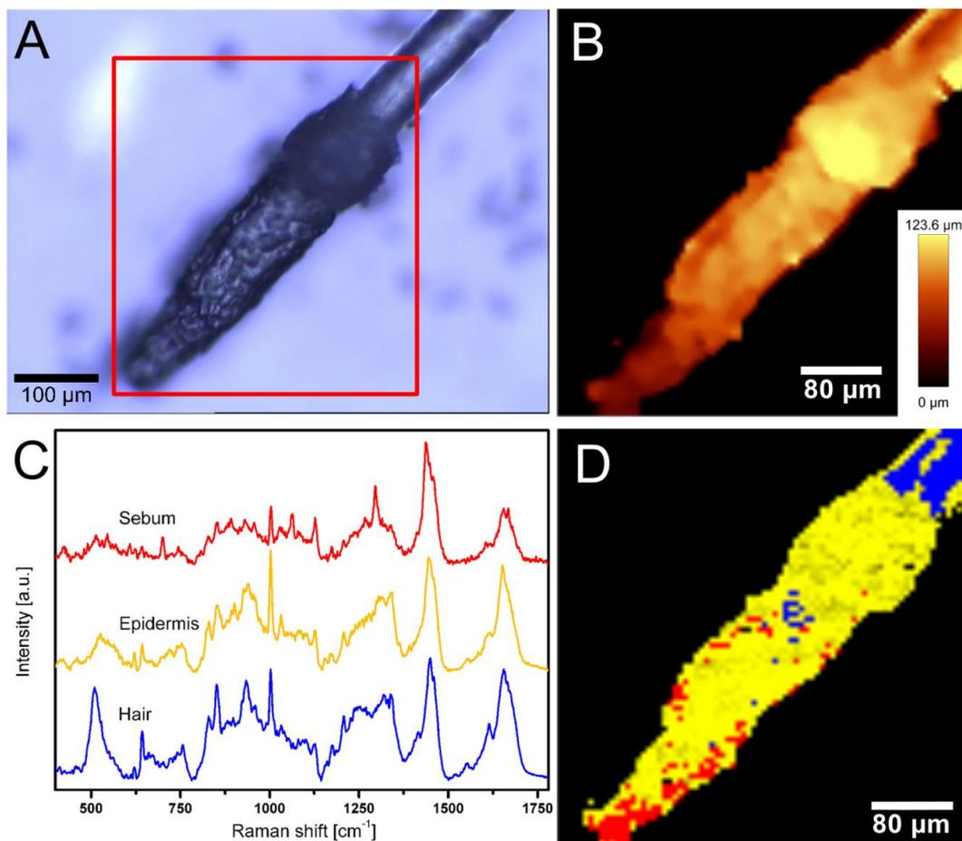
**Figure 5:** A Light microscopy picture of an excised hair follicle. B Surface topography map of the area indicated by the red rectangle in A. C Raman spectra of the individual chemical components in the hair follicle. D Raman map displaying the component distribution on the excised hair follicle. Reproduced with permission from (63).
