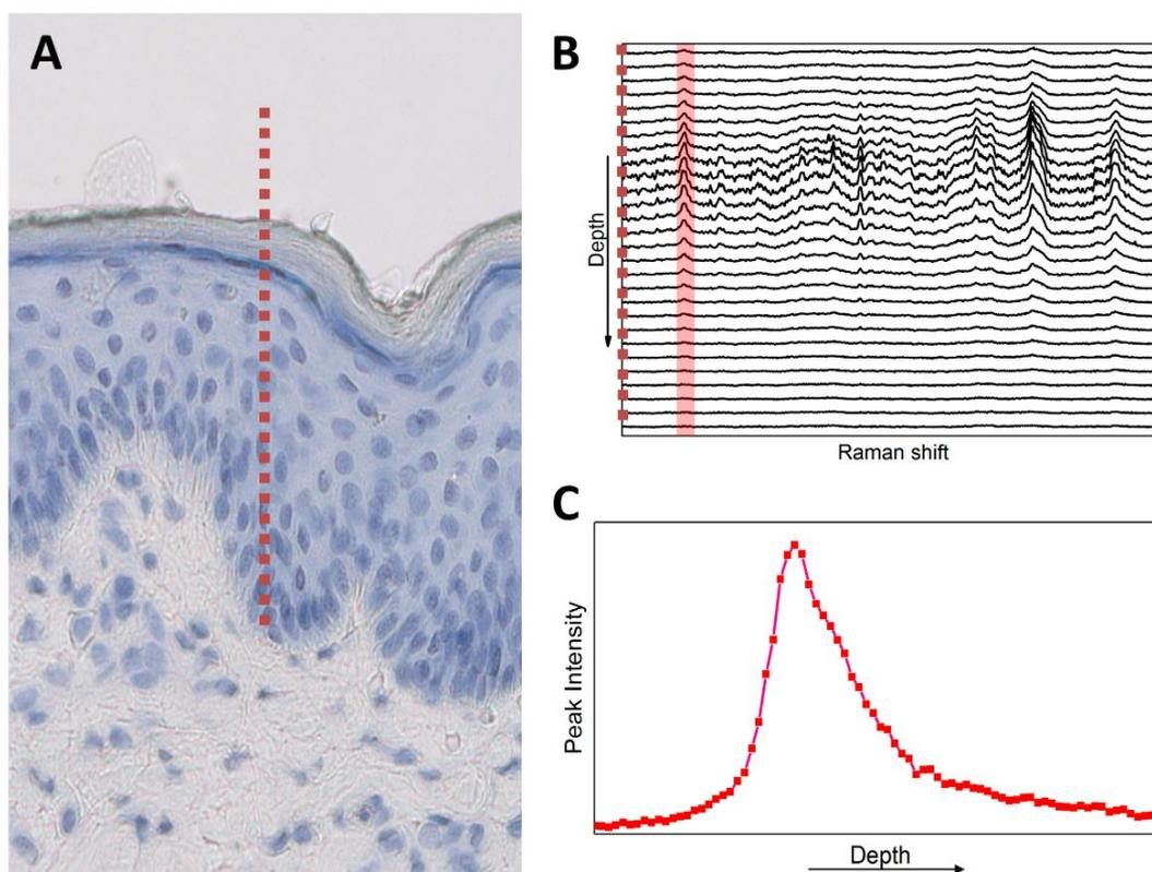
**Figure 3:** Schematic explanation of Raman signal attenuation. **A** Basic principle of depth profiling in skin. **B** Raman spectra recorded along the red line in A. **C** Intensity depth profile of a selected Raman peak highlighted in B. With ongoing depth, the Raman signal decays due to a reduced yield of collected photons. Reproduced with permission from (19).
