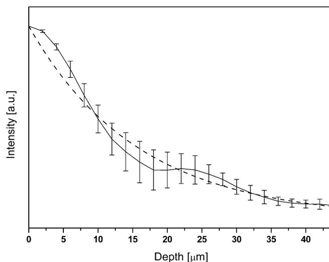
**Figure 6:** Raman mean drug intensity depth profile based on three skin surrogates (solid line mean  $\pm$  SD,  $n = 3$ ) and fitting function (dashed line). Reproduced with permission from (64).
