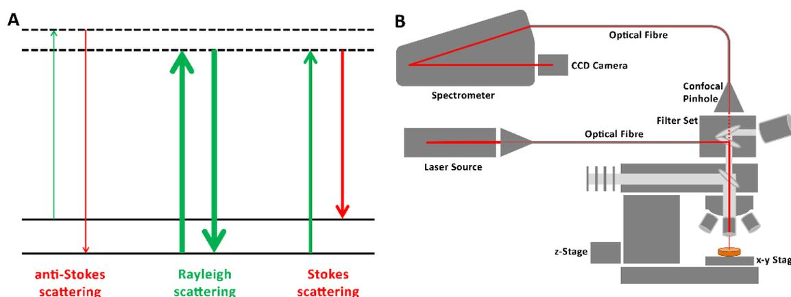
**Figure 1:** A Energy level diagram illustrating different types of scattering, line thickness corresponds with the probability of appearance. B Schematic of a confocal Raman microscopic setup, red lines indicate the way of excitation laser light and gathered Raman scattering. Reproduced with permission from (19).
