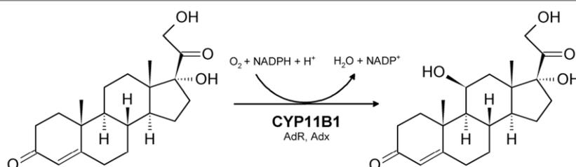
**Figure 1** Scheme of the CYP11B1-catalyzed 11 $\beta$ -hydroxylation of 11-deoxycortisol yielding cortisol. Electrons are transferred from NADPH via AdR and Adx to CYP11B1, which activates molecular oxygen and incorporates one oxygen atom into the steroid substrate by means of a hydroxylation in a regio- and stereoselective manner, while the other oxygen is reduced to water.
