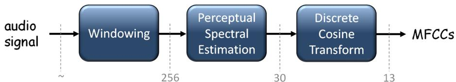
Figure 5.2: *Processing chain for Mel frequency cepstral coefficients.*
