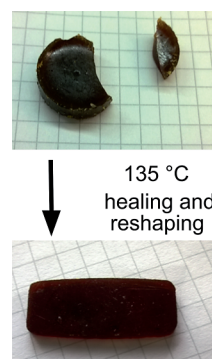
Figure 11. Rectangular specimen molded by healing and reshaping of M_2 -PDMS-cured Q_8M_8FAE_8 .
