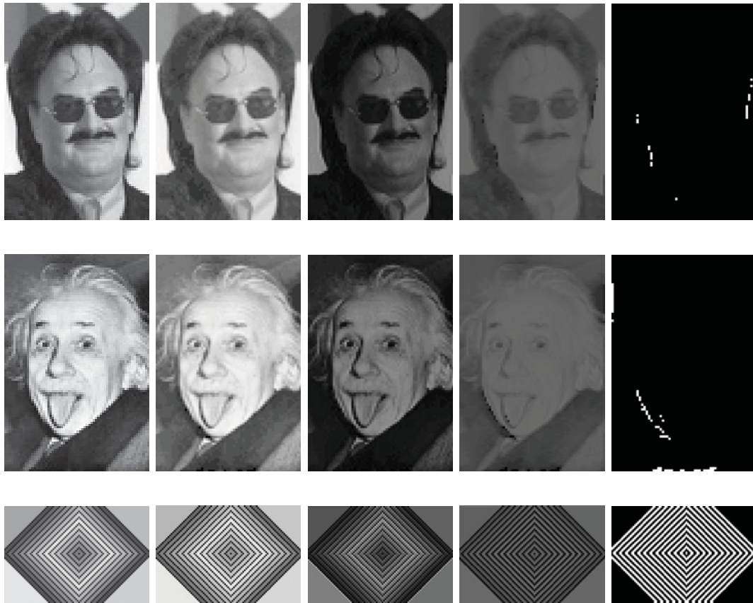
Figure 6.9: Visualisation of power saving and discharge for three test images. In each row from left to right: 5-bit source, linearised conventional driving injection times, SQC injection times, their difference reflecting the power saving, the discharge bitmap
