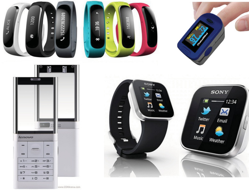
Figure 1.4: Recent products with PMOLED displays: Huawei Talkband [35], MD300 C2 Pulse Oximeter [49], Lenovo S800 mobile phone [45], Sony Ericsson Live View watch [70]
