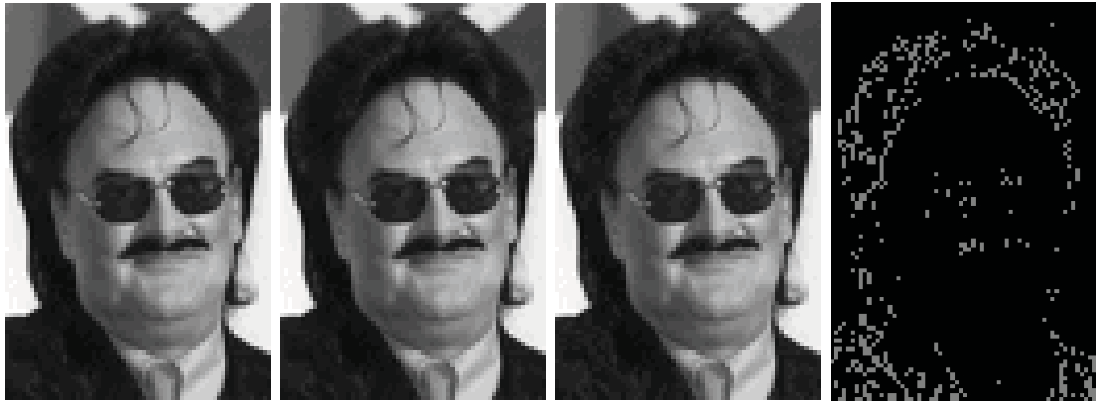
Figure 7.2: Image reconstruction in Matlab, from left to right: 5-bit source image, identical reconstruction with \Delta_{Lum,best} , SQC image and its 1-bit difference matrix with respect to the source
