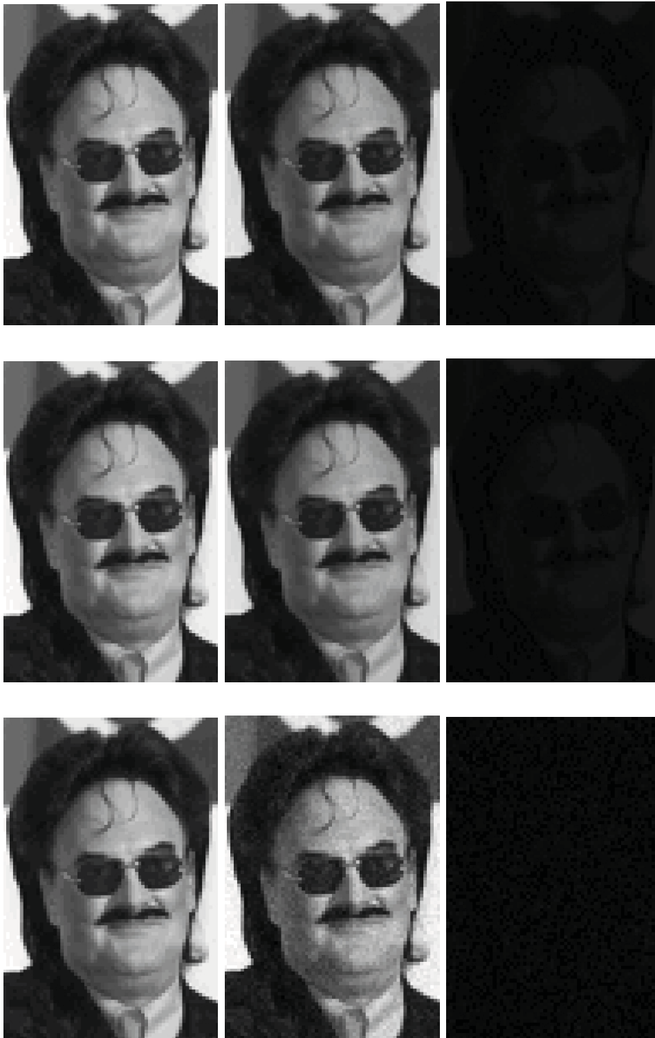
Figure 7.4: Parameter variation in Matlab. From left to right: 5-bit SQC image, SQC reconstruction with parameter variation, difference matrix. From top to bottom: 10% reduction of injection current, 10% reduction of cumulative capacitance, random reduction within 10% of state variables (voltages)
