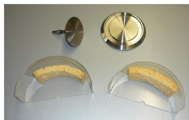
(b) Photograph of the cone-plate geometry C60/0.5°. It consists of a rotor (upper left part) and a cup (upper right part) as well as a plastic top cover with sponges (lower part).
