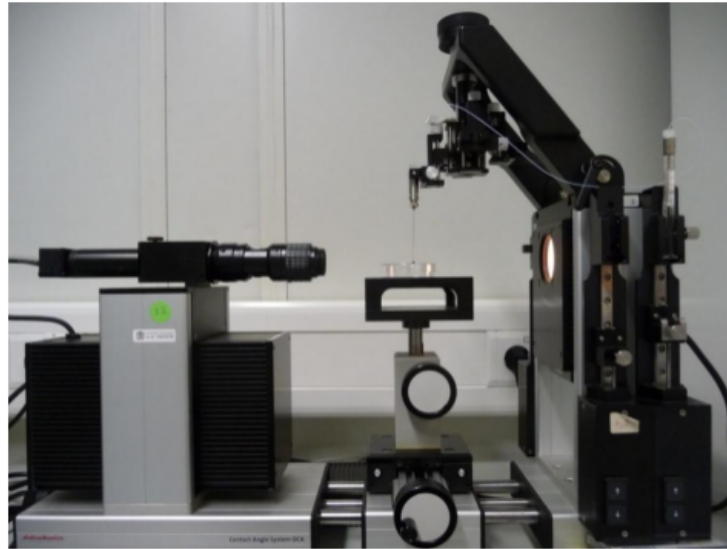
FIGURE 3.2: Our experimental setup with OCA20 instrument, used in measuring the contact angles of glass and basalt materials.
