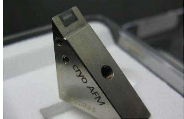
**Abb. 47:** Cryo AFM Messer v. DIATOME.
