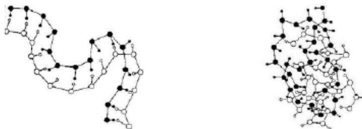
**Figure 4:** Limiting structures of polyelectrolyte complex precipitates. Left: Ladder model. Right: “Scrambled egg” model.
